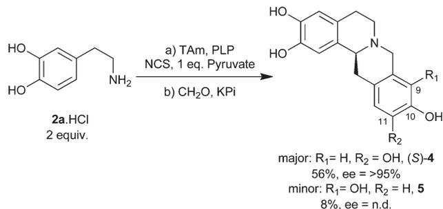
**Scheme 2** One-pot chemoenzymatic synthesis of (S)-**4** and (S)-**5**. Reaction conditions: (a) 20 mM **2**, 10 mM sodium pyruvate, 500  $\mu\text{g mL}^{-1}$  NCS and 20% v.v<sup>-1</sup> CV2025 lysate, 50 mM HEPES pH 7.5, 37 °C, 3 h. (b) 40 mM formaldehyde, 1 M sodium phosphate, pH 6, 30 min, 37 °C.
