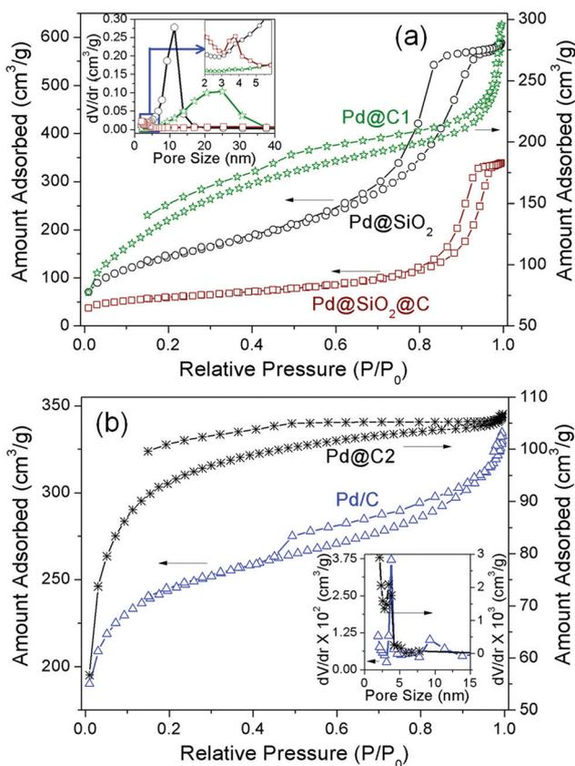
**Fig. 1** N<sub>2</sub> sorption isotherms and (inset) pore size distributions.
