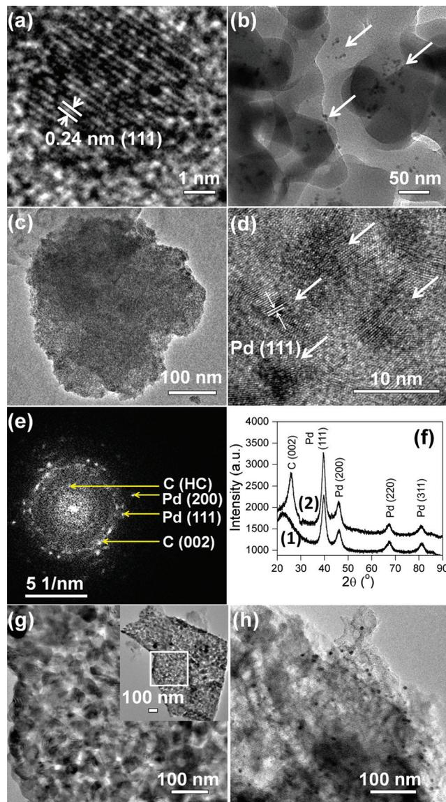
**Fig. 3** TEM images of (a) Pd NP, (b) Pd@SiO<sub>2</sub>, (c, d) Pd@C1. (e) SAED pattern of Pd@C1. HC denotes “high curvature”. (f) XRD patterns of (1) Pd@SiO<sub>2</sub> and (2) Pd@C1. TEM images of (g) Pd@C2, inset shows the entire matrix, and (h) Pd/C.
