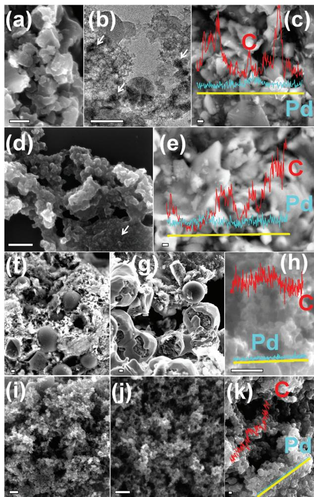
**Fig. 6** (a) FESEM image, (b) TEM and (c) elemental line scan of Pd@C1 after 200 cycles of MeOH EOx. (d) FESEM image and (e) elemental line scan of Pd@C1 after 300 cycles. FESEM images of Pd@C2 after (f) 200 and (g) 300 cycles. (h) Elemental line scan of Pd@C2 after 300 cycles. FESEM images of Pd/C after (i) 200 and (j) 300 cycles. (k) Elemental line scan of Pd/C after 300 cycles. Arrows indicate the agglomerated Pd NPs. All scale bars correspond to 200 nm.
