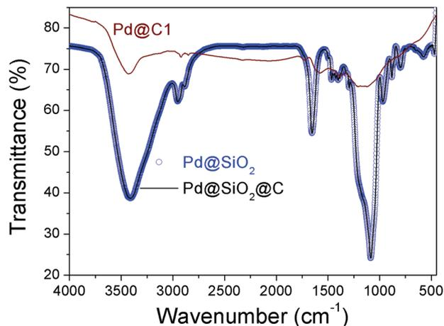
Fig. 4 FTIR spectra of Pd@SiO<sub>2</sub>, Pd@SiO<sub>2</sub>@C and Pd@C1.
