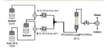
Fig. 3 Schematic representation of the set-up for segmented and continuous flow sulfoxidations catalysed by [PO<sub>4</sub>{WO(O<sub>2</sub>)<sub>2</sub>}<sub>4</sub>]@PIILP (2).
