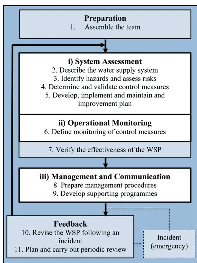
Fig. 2 How to Develop and Implement a WSP (11 modules) (adapted from Bartram *et al.*<sup>24</sup>).
