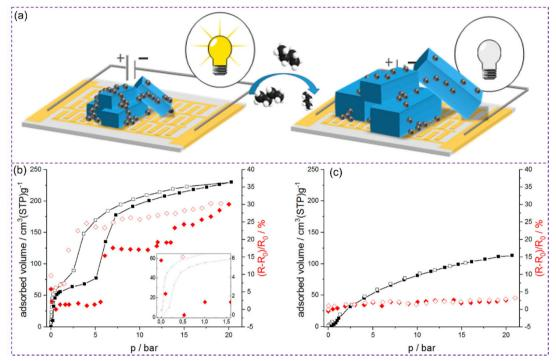
Fig. 17 (a) Schematic illustration of chemiresistive sensing of a usual MOF/conductive carbon hybrid. (b) and (c) CO2 and CH4 interaction induced resistance variations in CB/film hybrid. (Red diamonds = relative resistance change in the material and black squares = physisorption data; Closed symbols = adsorption; open symbols = desorption). Reproduced with permission from ref. 249 Copyright 2019, American Chemical Society.
