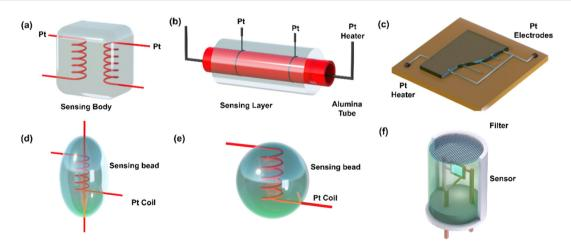
Fig. 5 Chemiresistive gas sensors are commonly built using various structures, including (a) sintered blocks, (b) thin alumina tube coatings, (c) screenprinted thick films, (d) small beads with coil and needle electrodes, (e) small beads with a single coil (heater and electrode), and (f) practical sensor elements assembled with metal caps and filters. Redraw the picture with permission from ref. 60 Copyright 2023 Elsevier.
