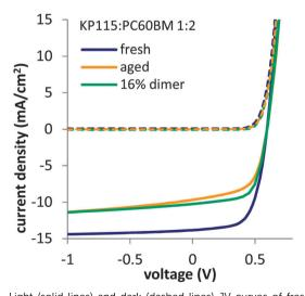
Fig. 1 Light (solid lines) and dark (dashed lines) JV curves of fresh and aged (120 h) KP115:PC60BM solar cells along with KP115:PC60BM solar cells containing 16% PC60BM dimers, added during cell production. PC60BM dimers were isolated using HPLC from photo-irradiated PC60BM films. The structure of KP115 (PDTSTzTz)<sup>3,33,34</sup> is given in the ESI.†
