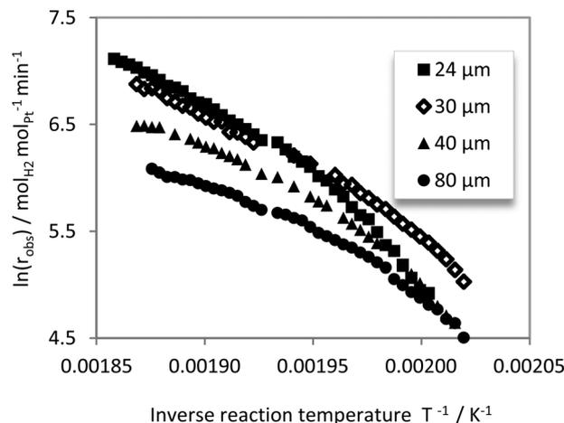
Fig. 8 Arrhenius plot derived from all experimental data obtained in this study: reaction temperatures: 224–261 °C; H<sub>2</sub>-NEC flow rate 0.6 mL min<sup>-1</sup>.
