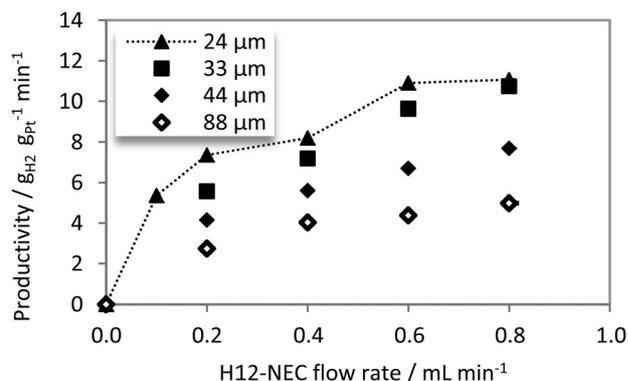
Fig. 5 Catalyst productivity as function of H12-NEC flow rate: reaction temperature: 260 °C  $\pm$  1 °C; catalysts: 24 μm, 33 μm, 44 μm, 88 μm; 30 catalyst spheres; Pt mass in reactor: 0.36–1.87 mg; productivity defined as gram H<sub>2</sub> released per gram Pt.
