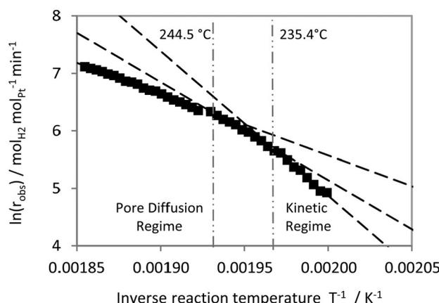
Fig. 9 Arrhenius plot for the 24 μm catalyst: reaction temperature: 224–261 °C; H<sub>2</sub>-NEC flow rate 0.6 mL min<sup>-1</sup>; active layer of catalyst: 24 μm; 30 catalyst spheres; Pt mass 0.36 mg; H<sub>2</sub>-yield <33%; constant slopes (kinetic vs. pore diffusion regime) are displayed as dashed lines.
