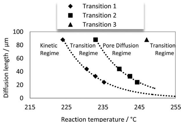
Fig. 11 Reaction regime map: reaction temperature: 224–261 °C; H12-NEC flow rate 0.6 mL min<sup>-1</sup>; catalysts: 24  $\mu\text{m}$ , 33  $\mu\text{m}$ , 44  $\mu\text{m}$ , 88  $\mu\text{m}$ ; 30 catalyst spheres; platinum mass: 0.36–1.87 mg.
