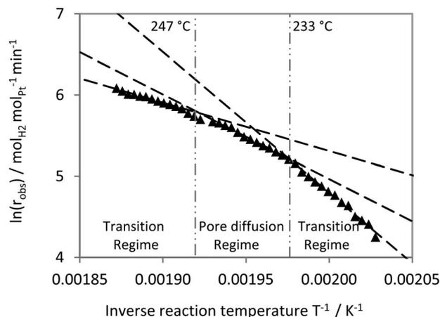
Fig. 10 Arrhenius plot for the 88 μm catalyst: reaction temperature: 224–261 °C; H<sub>2</sub>-NEC flow rate 0.6 mL min<sup>-1</sup>; active layer of catalyst: 88 μm; 30 catalyst spheres; Pt mass = 1.87 mg; H<sub>2</sub>-yield <33%; constant slopes (pore diffusion regime vs. transition regimes) are displayed as dashed lines.
