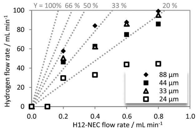
Fig. 4 Dehydrogenation of H12-NEC – effect of H12-NEC flow variation on hydrogen yields: reaction temperature: 260 °C; catalyst: 24 μm, 33 μm, 44 μm, 88 μm; 30 catalyst spheres; platinum mass between 0.36–1.87 mg.
