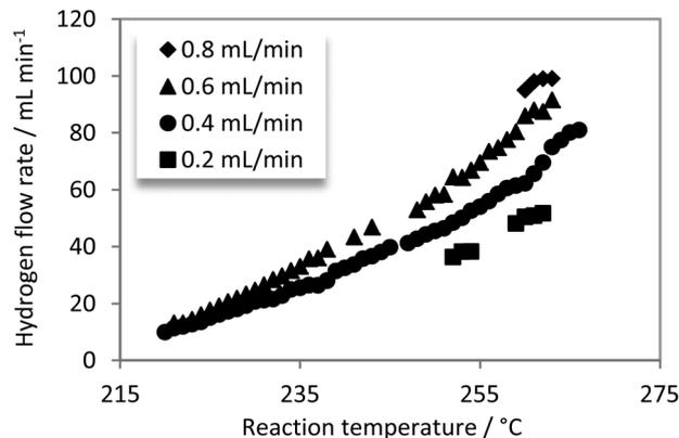
Fig. 3 Dehydrogenation of H12-NEC as a function of temperature: reaction temperature between 220 °C and 266 °C; H12-NEC flow rates between 0.2 mL min<sup>-1</sup> and 0.8 mL min<sup>-1</sup>; catalyst spheres with 33 μm coating thickness; 30 spheres applied  $\cong$  0.82 mg of total Pt.
