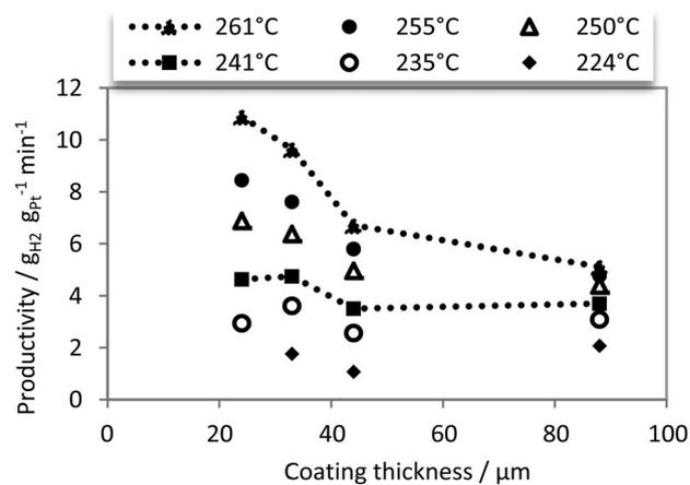
Fig. 7 Productivity as a function of diffusion length: reaction temperature: 224–261 °C; H12-NEC flow rate 0.6 mL min<sup>-1</sup>; catalysts: 24 μm, 33 μm, 44 μm, 88 μm; 30 catalyst spheres; Pt mass: 0.36–1.87 mg.
