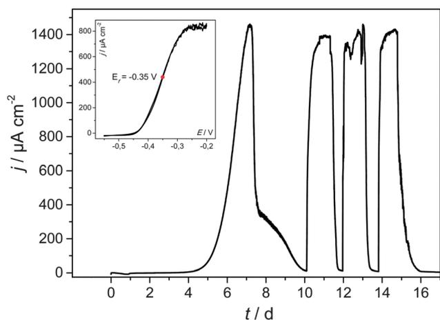
**Fig. 3** Main figure: cultivation and the resulting bioelectrocatalytic current generation of a secondary, acetate based electrochemically active biofilm at copper (copper sheet) in a model semi-batch experiment. The biofilm was cultivated in a half-cell setup under potentiostatic control. The electrode potential was  $-0.2$  V (vs. Ag/AgCl). Inset: cyclic voltammogram recorded under turnover conditions.
