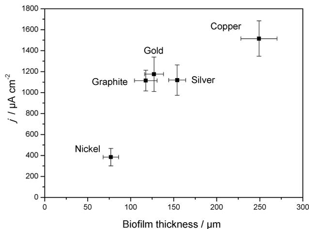
**Fig. 6** Correlation of the electrocatalytic current density of electrochemically active secondary biofilms cultivated on different electrode materials and of the biofilm thickness as determined *via* CLSM analysis.
