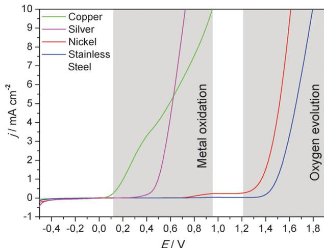
Fig. 7 Oxidative linear sweep voltammograms of selected metals (blank metal sheets), recorded in 0.1 M potassium nitrate solution. Scan rate  $1 \text{ mV s}^{-1}$ . Additional linear sweep voltammograms of copper and stainless steel, recorded in filtrated, primary wastewater, are illustrated in Fig. S6 (ESI<sup>†</sup>).
