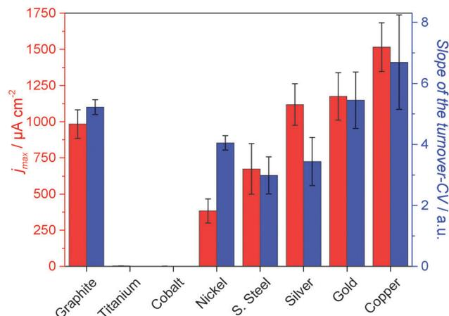
**Fig. 5** Electrochemical performance of electrochemically active secondary biofilms cultivated on different metals and on polycrystalline graphite. Red columns: average maximum current densities achieved during semi-batch cultivation (see Fig. 1 and 2); blue columns: mean values of the slopes of the turnover cyclic voltammograms of the respective biofilm electrodes. The error bars indicate the standard deviations. Substrate: 10 mM acetate, temperature 35 °C.
