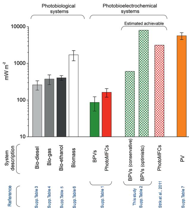
Fig. 7 Actual and theoretical power densities of photobiological, photobioelectrochemical and photovoltaic systems. Figures and means  $\pm$  standard errors have been calculated from published data and sources available in ESI Tables 2–7.†
