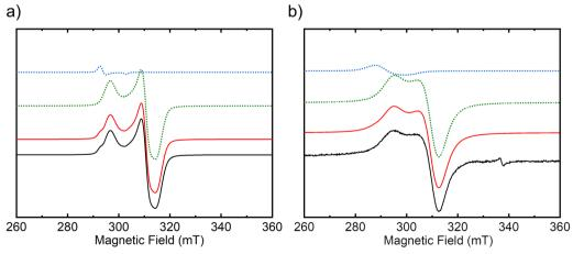
Fig. 4 Experimental (black lines) and simulated (red lines) X-band CW-EPR spectra of the  $Ni^{II}$ -NO adduct in Ni-MFU-4l- $NO_2$  formed upon NO adsorption and recorded at (a) 10 K and (b) 288 K. The simulation is composed of the sum of two different species A (dotted green line) and B (dotted blue line). The small signal around  $\sim 340$  mT corresponds to the radical.
