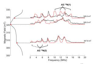
Fig. 5 Experimental (black) and simulated (red) X-band <sup>14</sup>N ENDOR spectra of Ni<sup>II</sup>-NO adduct in Ni-MFU-4l-NO<sub>2</sub> recorded at different magnetic field settings. The simulation of the <sup>14</sup>N(2) signal was obtained by using one of the DFT-computed set of Euler angles for the triazole <sup>14</sup>N. The ESE spectrum with the corresponding field positions at which the ENDOR spectra were taken is plotted on the left-hand side. All spectra were recorded at 10 K.
