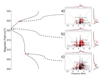
Fig. 6 Simulation (in red) of the X-band <sup>14</sup>N HYSCORE spectrum (in black) of Ni<sup>II</sup>-NO adduct in Ni-MFU-4l-NO<sub>2</sub> recorded at (a) 325.0 mT, (b) 320.8 mT, and (c) 309.0 mT. The ESE detected EPR signal of Ni<sup>II</sup>-NO is reported on the left side. Spectra were recorded at 10 K.
