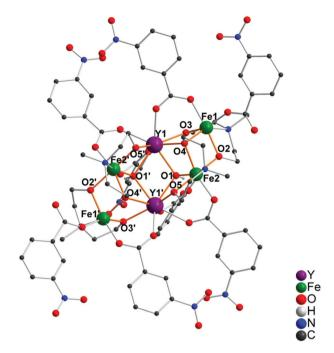
Fig. 1 Molecular structure of the coordination cluster in  $[Fe_4^{II}Y_2^{III}(\mu_3-OH)_2(mdea)_4(m-NO_2C_6H_4COO)_8]\cdot 3MeCN$  (1). Organic H atoms have been omitted for clarity.
