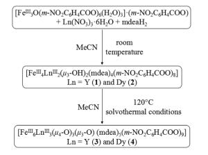
Scheme 1 A schematic representation of the synthetic routes of compounds 1–4. Details are given in the Experimental section.
