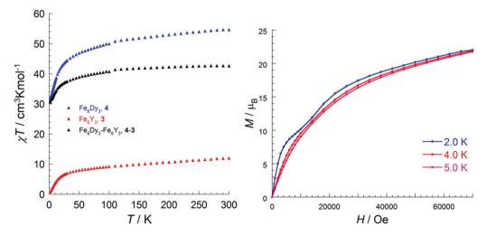
Fig. 4 (left) Temperature dependence of the  $\chi T$  product at 1000 Oe for 3 (red) and 4 (blue), and the adjusted  $\chi T$  vs. T plot for compound 4 with the data of compound 3 subtracted (black). (right) Field dependence of magnetization at low temperature for compound 4.
