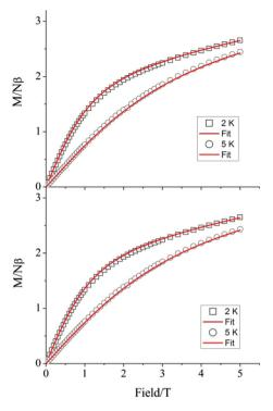
Fig. 4 Magnetisation of 1 as a function of applied field at (top) ambient pressure inside the pressure cell and (bottom) 1.6 GPa. Solid lines correspond to fits of the data, performed with the program Phi.
