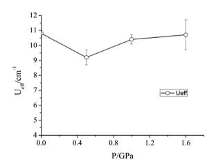
Fig. 5 Variation of the barrier to relaxation  $U_{\rm eff}$  of 1 under an applied do field of 2500 Oe as a function of pressure.
