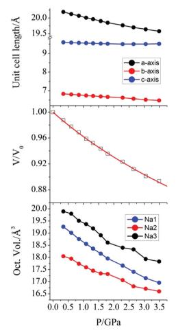
Fig. 2 (top) Variation of the crystallographic unit cell lengths in  $\bf 1$  as a function of applied pressure. (middle) Pressure dependence of the relative unit cell volume of  $\bf 1$ . The value at P=0 is taken from the original crystal structure determination,  $^{18}$  and the solid line is a fit to a Birch-Murnaghan equation of state. (bottom) The pressure dependence of the octahedral volume around the Na $^+$  ions in  $\bf 1$ .
