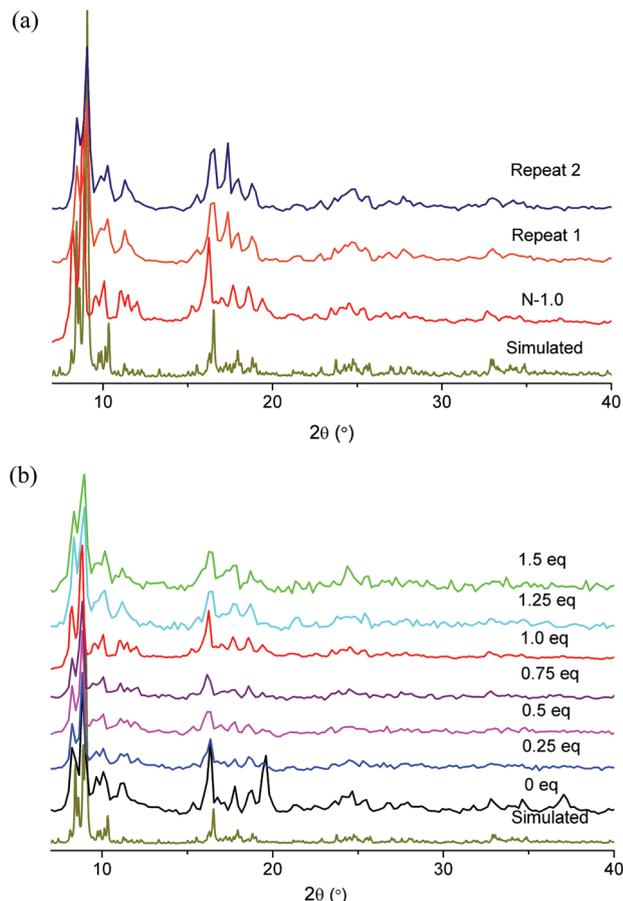
**Fig. 3** Powder X-ray diffractograms of (a) N-1.0 samples and (b) samples with other  $\text{HNO}_3$  equivalents in comparison with the simulated pattern (Cu-K $\alpha$  radiation).
