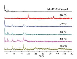
Fig. 5 PXRD of large-scale preparations of MIL-101(Cr) at different temperatures (diffractograms were recorded on a Bruker D8 Advance with DaVinci<sup>TM</sup>, Cu-K $\alpha$  radiation).
