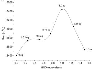
Fig. 2 (a)  $N_2$  adsorption–desorption isotherms of  $HNO_3$ -variable MIL-101(Cr); filled symbols are for adsorption, and empty symbols for desorption. (b) Plot of  $S_{BET}$  values  $versus\ HNO_3$  equivalents.
