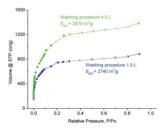
Fig. 6  $N_2$  sorption isotherms and BET surface areas of materials from large scale synthesis and different washing procedures. The noted procedure "1.5 L – blue" ("4.5 L – green") refers to washing with 1.5 L (4.5 L) DMF – separation – 1.5 L (4.5 L) ethanol – separation – 1.5 L water; see the Experimental section for details of the 4.5 L procedure.
