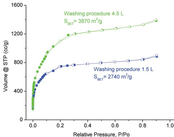
**Fig. 6** N<sub>2</sub> sorption isotherms and BET surface areas of materials from large scale synthesis and different washing procedures. The noted procedure "1.5 L – blue" ("4.5 L – green") refers to washing with 1.5 L (4.5 L) DMF – separation – 1.5 L (4.5 L) ethanol – separation – 1.5 L water; see the Experimental section for details of the 4.5 L procedure.
