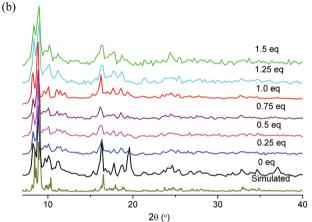
Fig. 3 Powder X-ray diffractograms of (a) N-1.0 samples and (b) samples with other HNO<sub>3</sub> equivalents in comparison with the simulated pattern (Cu-Kα radiation).
