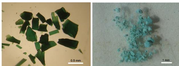
Fig. 8 Image of MIL-101(Cr) with acetic acid (8.3 equivalents, 220 °C) (left) and HNO<sub>3</sub> (N-1.0) (right) as a modifier.
