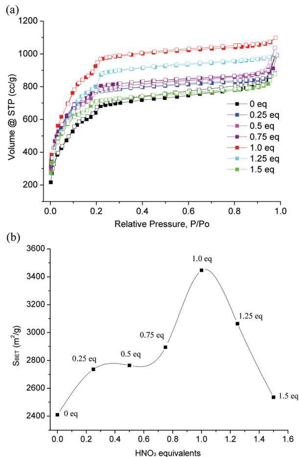
**Fig. 2** (a) N<sub>2</sub> adsorption–desorption isotherms of HNO<sub>3</sub>-variable MIL-101(Cr); filled symbols are for adsorption, and empty symbols for desorption. (b) Plot of S<sub>BET</sub> values versus HNO<sub>3</sub> equivalents.
