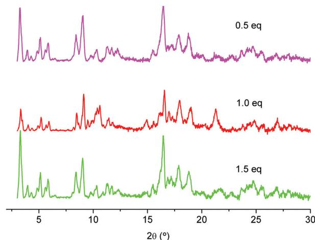
**Fig. 7** PXRD of large-scale preparations of MIL-101(Cr) with different equivalents of HNO<sub>3</sub>. (PXRD data were recorded on a Bruker D8 Advance with DaVinci™, Cu-K $\alpha$  radiation).
