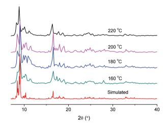
Fig. 10 Powder X-ray diffractograms of "seeded" samples with 8.3 eq. of acetic acid at different temperatures compared with the simulated MIL-101(Cr) pattern.
