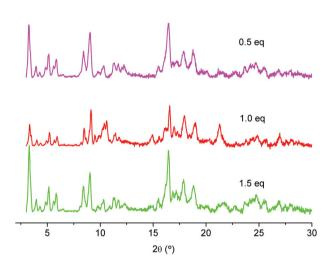
Fig. 7 PXRD of large-scale preparations of MIL-101(Cr) with different equivalents of HNO<sub>3</sub>. (PXRD data were recorded on a Bruker D8 Advance with DaVinci<sup>TM</sup>, Cu-K $\alpha$  radiation).
