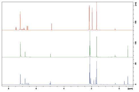
Fig. 1 <sup>1</sup>H NMR spectra of 1 (top), MeLZnMe (middle) and the reaction of 1 and Me<sub>2</sub>Zn (bottom), demonstrating the substitution of only one MeLZn moiety by a MeZn unit.
