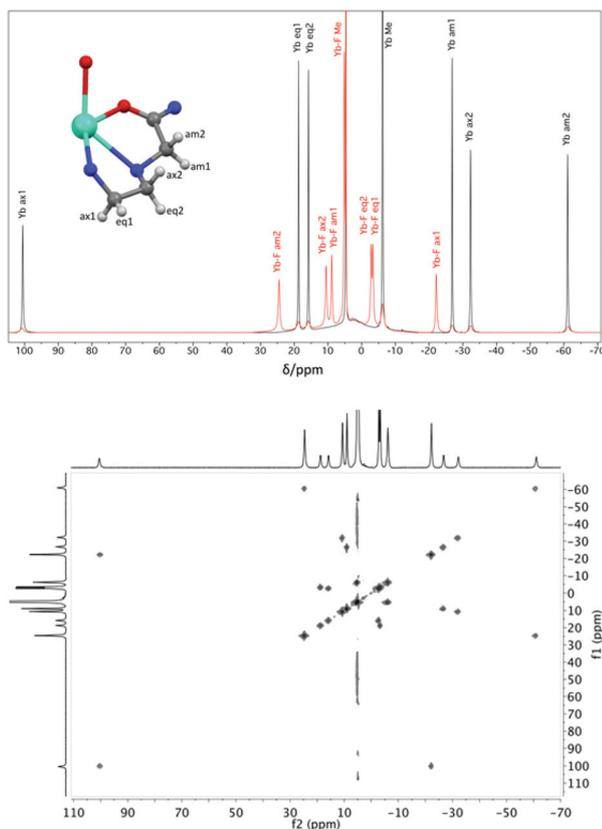
**Fig. 3** Top:  $^1\text{H}$  NMR spectra (400 MHz, 298 K,  $\text{D}_2\text{O}$ ) of YbDTMA in the absence (black) and presence (red) of an excess of sodium fluoride, with assignments based on the labelled portion of the complex shown (using DyDTMA crystal structure<sup>12</sup>). Bottom: EXSY spectrum of YbDTMA with fluoride at 298 K with a mixing time of 1 ms at 500 MHz.
