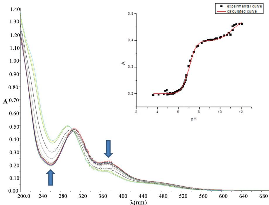
Fig. 4 UV-vis spectra recorded for 0.1 mM  $[\text{Pd}(\text{DPENim}^{\text{iPr}})(\text{H}_2\text{O})_2]^{2+}$  in the pH range 2 to 12 at 25 °C. Insert: plot of absorbance vs. pH at 260 nm (experimental curve and calculated curve).
