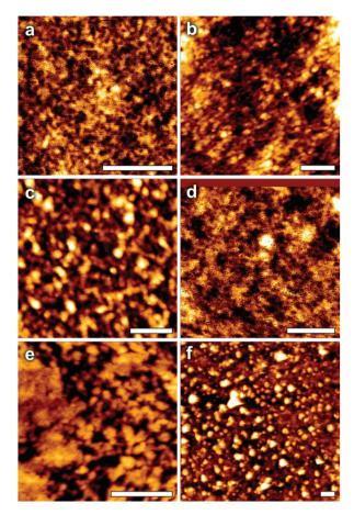
Fig. 6 AFM height images of bismuth clusters dried onto mica substrates, where values refer to approximate cluster sizes obtained from analysis of the AFM image: (a)  $K[Bi(BHA)_2]$  9: 3.5 nm; (b)  $[Bi(BPHA)_3]$  7: 4 nm; (c)  $[Bi(H-SHA)_3]$  1: <0.5 nm; (d) [Bi(AHA)(H-AHA)] 5: 5 nm; (e)  $[Bi(MFHA)_3]$  3: 1.8 nm; (f) [Bi(BHA)(H-BHA)] 6: <0.5 nm. The white scale bar in each image represents 200 nm.
