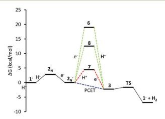
Fig. 6 Energy coordinate diagram for alternative paths to PCET. Red: 2<sub>N</sub><sup>-</sup> is first protonated (7), then reduced at the Ni centre; green reduced to 6, and proton migration, 8; blue: concerted PCET.
