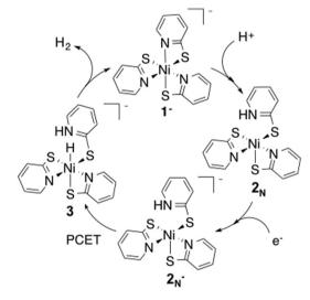
Fig. 1 Proposed catalytic cycle for proton reduction by  $[Ni(PyS)_3]^-$ ,  $1^-$ . Cation omitted.
