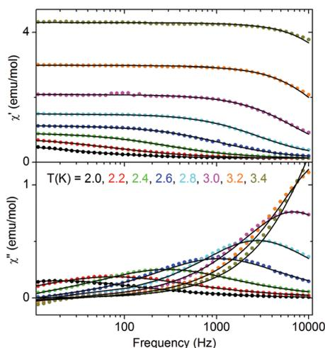
Fig. 9 Frequency dependent AC susceptibility for 2 measured at various temperatures. Solid lines are fits with the generalized Debye model.
