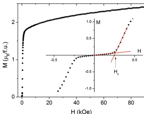
Fig. 6 Magnetization vs. field measured at  $T = 2.0$  K for 2. The inset magnifies the low-field region and shows the way of critical field determination.
