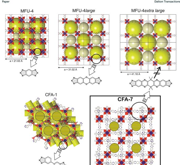
Fig. 2 An overview of different bistriazolate frameworks of the MFU-4 family with Kuratowski-type secondary building units. MFU-4, MFU-4l and the DFT-calculated MFU-4XL are representatives of the MFU-4 family which crystallize in a cubic crystal system, whereas CFA-1 exhibits a trigonal crystal lattice. The interpenetrated CFA-7 framework described herein crystallizes in the trigonal space group  $R\bar{S}m$  (no. 166).
