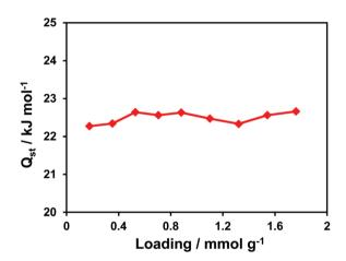
Fig. 15 Loading-dependent isosteric heat of CO<sub>2</sub> adsorption in CFA-7.
