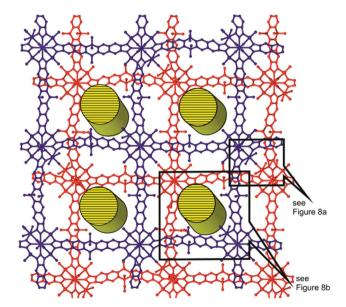
Fig. 7 Interpenetrated structure of CFA-7. In yellow the apparent pore aperture of the channels of the network is given (calculated with the Poreblazer software<sup>17</sup>).
