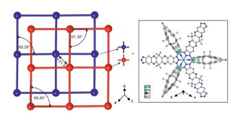
Fig. 9 Schematic representation of the two-fold interpenetrated CFA-7 networks (left) and its SBU with the disordered organic linker in *c*-direction (right, positional disorder of two parts of the ligand with the occupancy of 0.5/0.5, one part shown in ellipses).
