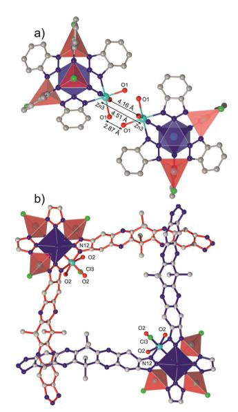
Fig. 8 Coordination environments of Zn ions in the Kuratowski-type secondary building units of CFA-7; (a) staggered arrangement of six water ligands from two different SBUs; (b) peripheral Zn ions which are coordinated to three N-atoms and one Cl-atom or to three N-atoms and three O-atoms.
