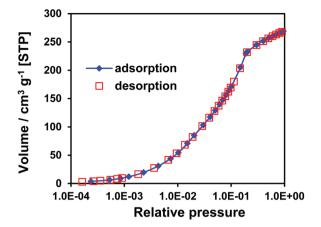
Fig. 14 CO<sub>2</sub> adsorption/desorption isotherm for CFA-7 at 194.7 K.
