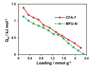
Fig. 16 Loading-dependent isosteric heats of H<sub>2</sub> adsorption in CFA-7 and MFU-4I.
