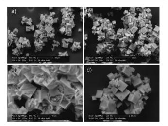
Fig. 12 SEM micrographs of CFA-7: (a) cubic CFA-7 crystals after the postsynthetic metal exchange with CoCl<sub>2</sub>; (b) exchange with NiCl<sub>2</sub>; (c) metal exchange with MnCl<sub>2</sub>; (d) crystals after exchange with Cu(ClO<sub>4</sub>)<sub>2</sub>.
