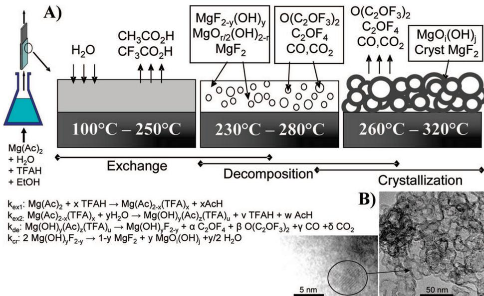
**Fig. 1** (A) Scheme representing the deposition of porous MgF<sub>2</sub> films on Si substrates by the TFA route; (B) TEM images showing the vesicle-like structures of the film prepared at 10 °C min<sup>-1</sup> under a dry atmosphere. Reprinted with permission from ref. 6a. © 2015 American Chemical Society.
