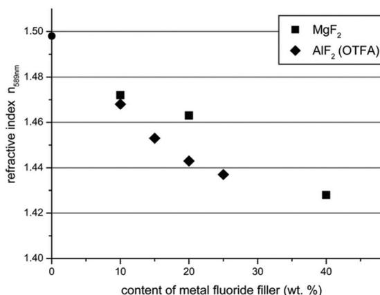
**Fig. 21** Photograph of a representative composite sample with 10 wt%  $\text{MgF}_2$  in a PolyHEMA matrix as bulk material (left) and refractive indices of thin film coatings based on magnesium and aluminium fluoride with different filler contents in a matrix of Poly(1,4-BDDMA) determined by ellipsometry (right). Reproduced from ref. 56 with permission of The Royal Society of Chemistry.
