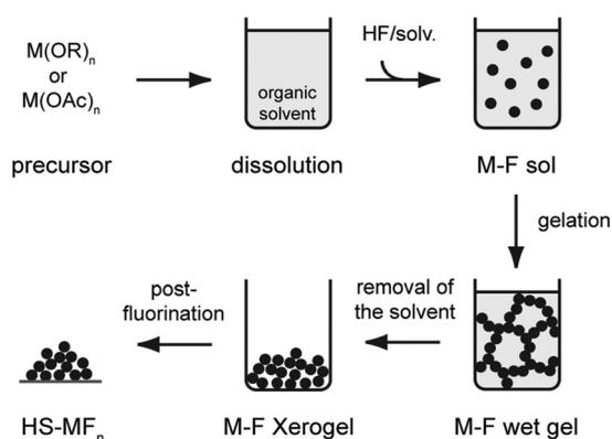
**Scheme 2** Illustration of the fluorolytic sol-gel synthesis starting from a metal alkoxide or carboxylate.
