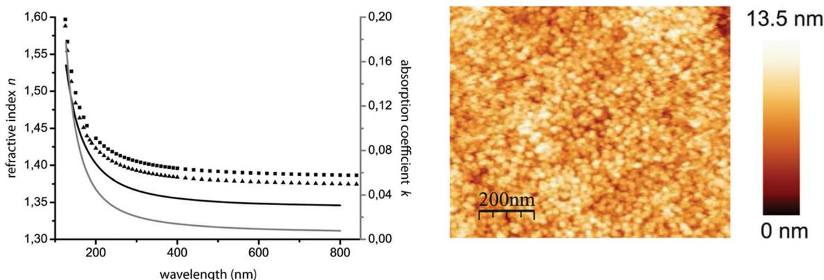
Fig. 18 Comparison of the refractive index  $n$  and absorption coefficient  $k$  of a  $\text{MgF}_2$ -film prepared from a 0.15 M sol on a silicon wafer (solid lines) with values from literature (squares: e-pol and triangles: o-pol) for bulk  $\text{MgF}_2$ <sup>54</sup> between 150 nm and 800 nm (left). AFM image of a three step coated  $\text{MgF}_2$ -layer on a silicon wafer calcined at 300 °C. Reproduced from ref. 53b (right) with permission of Elsevier.
