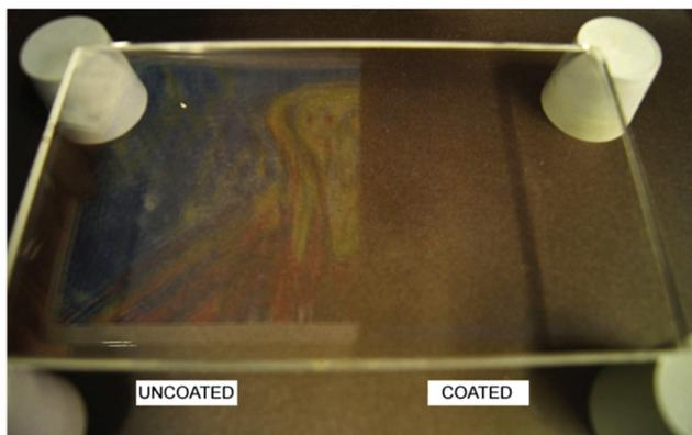
**Fig. 19** Glass substrate coated by  $\text{MgF}_2$  (right) whereas the left side is untreated. An image is shown above the glass and the mirror (left) or non-mirror (right) effect of each area while taking a picture from above can be seen.
