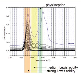
Fig. 13 CO IR difference spectra on sol gel derived HS-AlF<sub>3</sub>.  $\nu$ (CO) = 2150 cm<sup>-1</sup> - physisorbed CO;  $\nu$ (CO) = 2175 cm<sup>-1</sup> - medium strong Lewis acid sites;  $\nu(CO) = 2240 - 2220 \text{ cm}^{-1} - \text{very strong Lewis acid sites}$ . Reproduced from ref. 26 with permission of the Royal Society of Chemistry.
