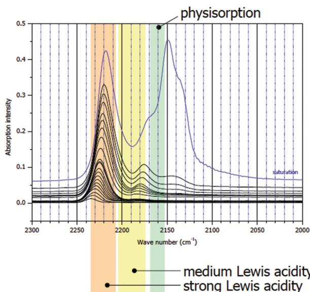
**Fig. 13** CO IR difference spectra on sol gel derived HS- $\text{AlF}_3$ .  $\nu(\text{CO}) = 2150 \text{ cm}^{-1}$  – physisorbed CO;  $\nu(\text{CO}) = 2175 \text{ cm}^{-1}$  – medium strong Lewis acid sites;  $\nu(\text{CO}) = 2240\text{--}2220 \text{ cm}^{-1}$  – very strong Lewis acid sites. Reproduced from ref. 26 with permission of the Royal Society of Chemistry.
