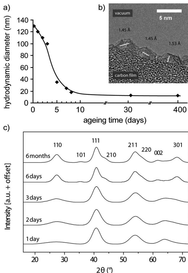
**Fig. 12** Hydrodynamic diameter (a) and X-ray diffraction patterns (c) of the  $\text{MgF}_2$  particles in the sol at different ageing stages, and HR-TEM image visualising  $\text{MgF}_2$  primary particles from phosphonic acid stabilized sol (b). Reproduced from ref. 29b with permission of the Royal Society of Chemistry.
