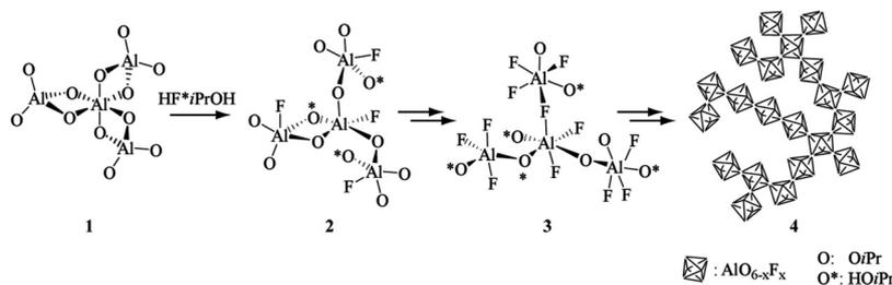
**Scheme 3** Schematic representation of the formation of highly distorted nanoscopic aluminium fluoride by reacting aluminium isopropoxide with anhydrous hydrogen fluoride in isopropanol as the solvent.
