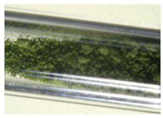
Fig. 1 A sample of extremely moisture-sensitive green  $Ag(i)_2Ag(i)(SbF_6)_4$  enclosed in a prefluorinated 0.3 mm quartz capillary.
