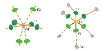
Fig. 3 The 4 + 4 coordination sphere of silver and the closest contacts to the  $[SbF_6]^-$  anion in the crystal structure of  $Ag_3(SbF_6)_4$  (dashed lines: longer  $Ag1\cdots F2$  contacts; outlined bonds: shorter Sb1-F2 distances; thermal ellipsoids are drawn at the 40% probability level).
