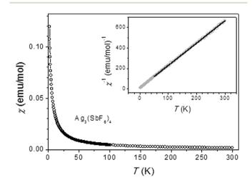
Fig. 7 Temperature-dependent susceptibility  $\chi(T)$  and inverse susceptibility  $\chi^{-1}(T)$  (inset) of Ag<sub>3</sub>(SbF<sub>6</sub>)<sub>4</sub> as measured in a magnetic field H=1000 Oe. The full line in the inset is a fit with the Curie–Weiss law.
