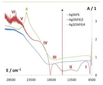
Fig. 8 Electronic absorption spectra of Ag<sub>3</sub>(SbF<sub>6</sub>)<sub>4</sub>, Ag(SbF<sub>6</sub>)<sub>2</sub>, and AgSbF<sub>6</sub> in the vis-NIR region. The 5-8.5k cm<sup>-1</sup> region is predominated by instrumental artefacts and it has not been shown. Starlet marks the artefact, while Roman numbers and # indicate bands which are dis-
