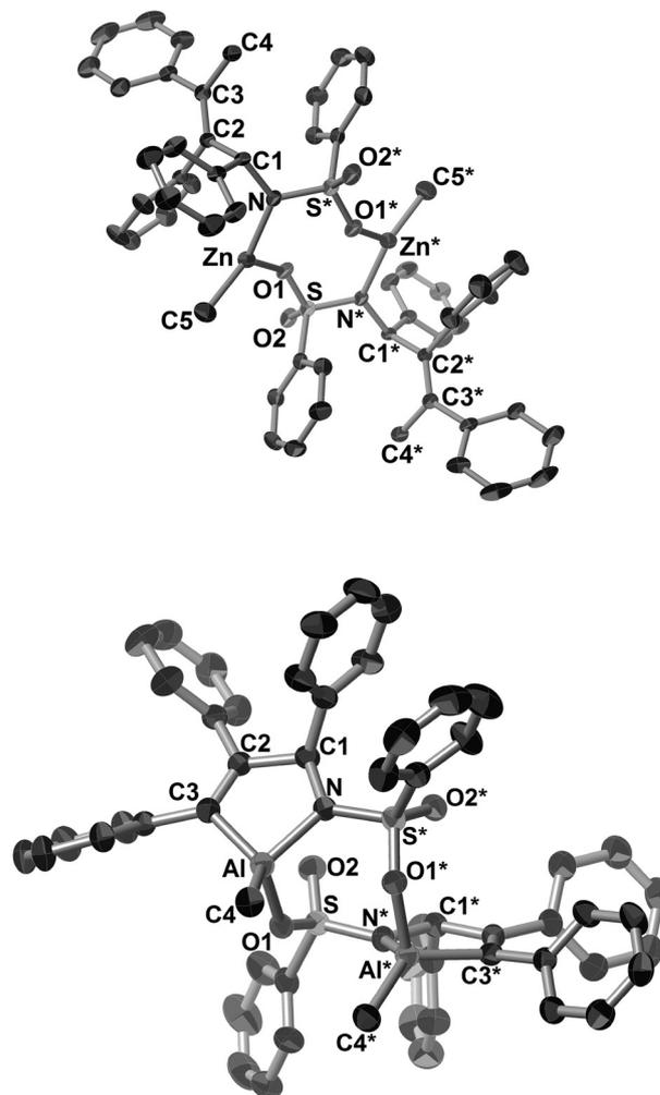
**Fig. 5** ORTEP drawings of **12aa** (a) and **13aa** (b) with thermal ellipsoids at the 30% probability level. H atoms and the solvated molecule (toluene) in **13aa** have been omitted for clarity. Symmetry transformation used to generate equivalent atoms  $\text{S}^*$  for **12aa**: 2 - X, Y, 2 - Z, for **13aa**: 2 - X, Y, 0.5 - Z.
