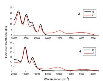
Fig. 7 Near-IR (NIR) absorption spectra for 3 (top) and 4 (bottom) and their cations in 0.1 M [Bu<sub>4</sub>N][PF<sub>6</sub>]/DCM using a SEC cell.
