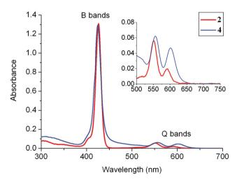
Fig. 2 Absorption spectra (in DCM) of the new dyads 3 and 4 (10<sup>-5</sup> M) at room temperature. The corresponding precursors 1 and 2 are included for comparison.
