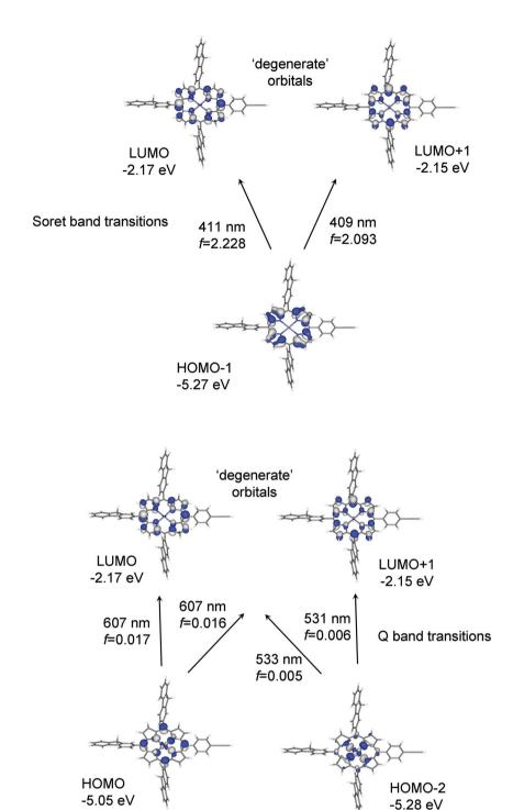
Fig. 11 Orbitals involved in the B-(Soret) and Q-bands for 2 based on TD-DFT data with computed wavelength and oscillator strength (f) listed for each transition.
