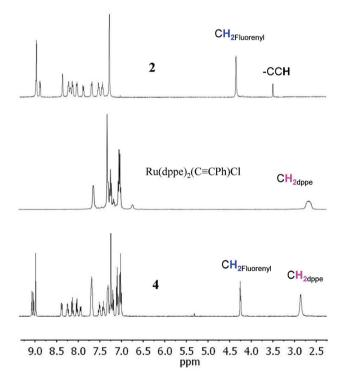
Fig. 1  $^{1}$ H NMR spectra (400 MHz, in CDCl<sub>3</sub>) of zinc porphyrin 2, Ru (dppe)<sub>2</sub>(C $\equiv$ CPh)Cl and the new dyad 4.
