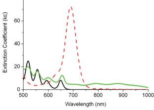
Fig. 5 UV-visible absorption spectra for 1 and its oxidised and reduced species in 0.1 M  $[Bu_4N][PF_6]/DCM$  using a thin-layer spectroelectrochemistry (SEC) cell.
