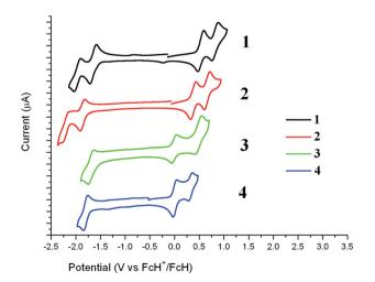
Fig. 4 Cyclic voltammograms for 1–4 in DCM in the presence of 0.1 M  $[Bu_4N][PF_6]$  as the supporting electrolyte. The current is scaled at 5  $\mu$ A between each tick mark.
