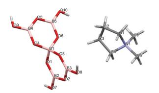
Fig. 3 Drawing of the structure of  $[C_4H_8NMe_2][B_5O_6(OH)_4]$  (2) showing the atomic numbering scheme.
