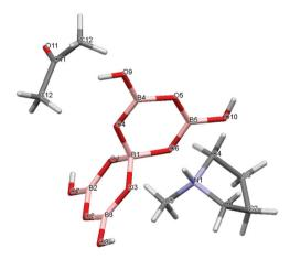
Fig. 4 Drawing of the structure of  $[C_4H_8NMeH][B_5O_6(OH)_4]\cdot 1/2C_3H_6O$  (3·1/2CH<sub>3</sub>COCH<sub>3</sub>), showing the atomic numbering scheme.
