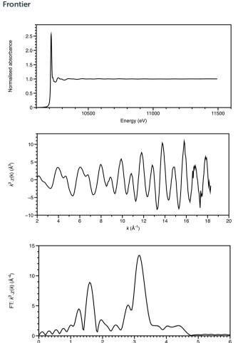
**Fig. 1** W L<sub>III</sub>-edge XAFS of  $(NBu_4)_2[W_6O_{19}]$  showing the normalised absorption spectrum (top), the  $k^3$ -weighted EXAFS (middle) and the Fourier transform (bottom). Data recorded on B18 of the Diamond Light Source.
