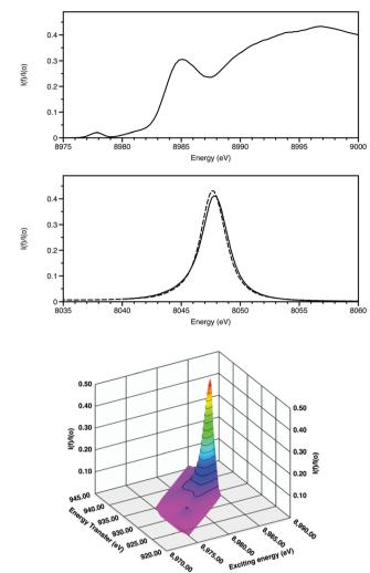
Fig. 2 Cu K-edge XANES of CuO showing the HERFD spectrum (top),  $K\alpha_1$  emission spectra of CuO (solid) and Cu (dashed) with the exciting energy above the absorption edge (middle) and  $K\alpha_1$  RIXS (bottom). Energy transfer = Exciting energy – emission energy. Data recorded on 120 of the Diamond Light Source.
