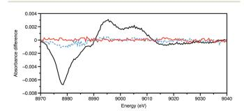
Fig. 3 Cu K-edge XTA of  $[Cu(2,9-Me_2-phen)_2]^+$  in MeCN (20 mM) showing the data 5 ns before laser pulse (450 nm) (red), during the pulse (black), and 5 ns after (blue). Data recorded on ID24 of the ESRF.
