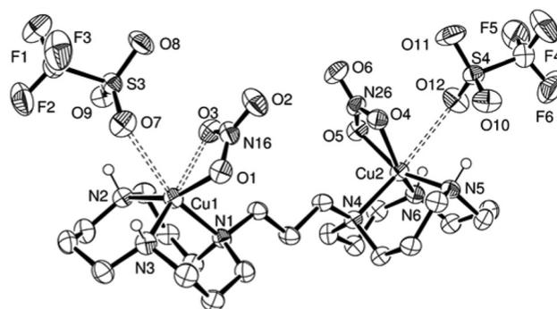
Fig. 1 ORTEP representation of **L3Cu<sub>2</sub>(NO<sub>3</sub>)<sub>2</sub>(TfO)<sub>2</sub>·(CH<sub>3</sub>OH)<sub>0.7</sub>(H<sub>2</sub>O)<sub>0.3</sub>** at 50% probability. Non-acidic hydrogen atoms and solvent molecules were omitted for clarity.
