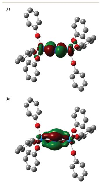
Fig. 4 Three dimensional representations of the  $\alpha$  HOMO–8 (a) and  $\alpha$  HOMO–1 (b) molecular orbitals of  $[Pa(OPh)_3]_2(\mu-\eta^2:\eta^2-N_2).$  Isovalue = 0.04. Hydrogen atoms are omitted for clarity. Orbital compositions (Mulliken analysis, %) are 18% Pa f, 12% Pa d, 50% N p and 22% Pa f, 8% Pa d, 68% N p respectively.
