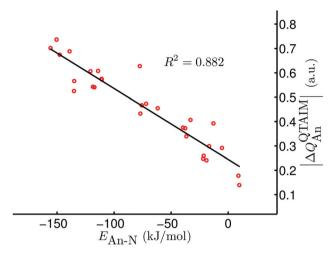
Fig. 5  $|\Delta Q_{An}^{QTAIM}|$  vs.  $E_{An-N}$  for  $[AnX_3]_2(\mu-\eta^2:\eta^2-N_2)$  (An = Th-Pu; X = F, Cl, Br, Me, H). Data for  $[Np(OPh)_3]_2(\mu-\eta^2:\eta^2-N_2)$  are not included.
