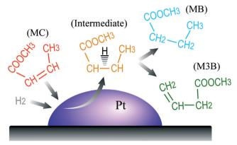
Fig. 8 Proposed reaction pathway for MC hydrogenation to form MB and M3B over the Pt/Al<sub>2</sub>O<sub>3</sub> catalyst.
