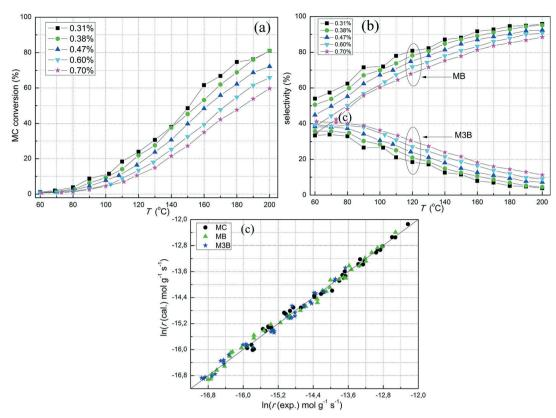
Fig. 4 (a) MC conversion and (b) selectivity of MC hydrogenation over the Pt/Al<sub>2</sub>O<sub>3</sub>-500 catalyst at various MC concentrations. (c) Experimental reaction rates of MC hydrogenation on the catalyst versus the calculated values by using the power-law model. Experimental conditions: 20 mg,  $p_{\rm H_2}$  = 2.58% and GHSV = ~240 000 h<sup>-1</sup>.
