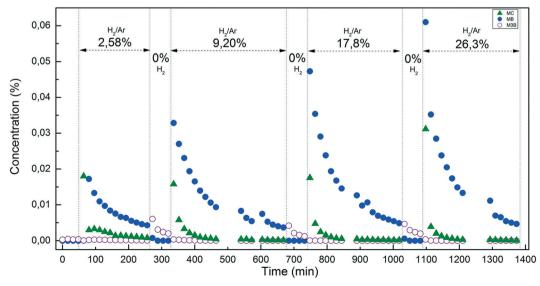
Fig. 6 Transient experiments over the Pt/Al<sub>2</sub>O<sub>3</sub>-500 catalyst under isothermal conditions at 190 °C by switching the gas feed between 0.46% MC and different H2 partial pressures.
