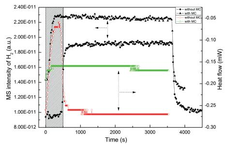
Fig. 7 H<sub>2</sub> chemisorption on the Pt/Al<sub>2</sub>O<sub>3</sub>-500 catalyst without and with MC at 25 °C.
