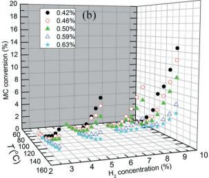
Fig. 9 MC conversions over the (a) Pt/Al<sub>2</sub>O<sub>3</sub>-500 and (b) Pt/Al<sub>2</sub>O<sub>3</sub>-700 catalysts at different MC and H2 partial pressures and reaction temperatures.
