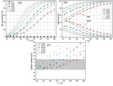
Fig. 5 (a) MC conversion, (b) selectivity and (c) carbon balance of MC hydrogenation on the Pt/Al<sub>2</sub>O<sub>3</sub>-500 catalyst at different H<sub>2</sub> concentrations. Experimental conditions: 20 mg catalyst,  $P_{\rm MC}$  = 0.60% and GHSV = ~240 000 h<sup>-1</sup>.
