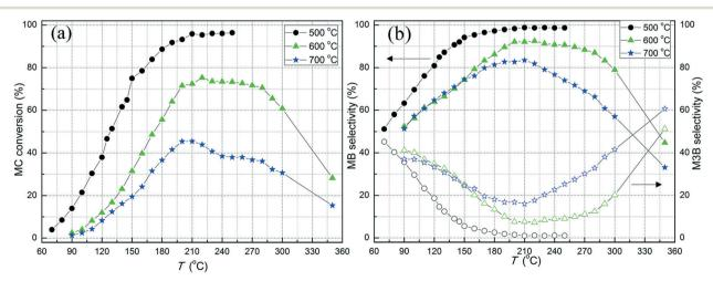
Fig. 2 (a) MC conversion and (b) selectivity as a function of reaction temperature for MC hydrogenation over the Pt/Al<sub>2</sub>O<sub>3</sub> catalysts calcined at different temperatures. Experimental conditions: 20 mg catalyst,  $p_{MC} = 0.63\%$ ,  $p_{H_2} = 4.60\%$  and GHSV = ~240 000 h<sup>-1</sup>.
