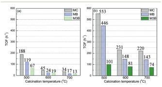
Fig. 3 Comparison of TOFs of the three Pt/Al<sub>2</sub>O<sub>3</sub> catalysts towards MC hydrogenation at (a) 90 and (b) 120 °C.
