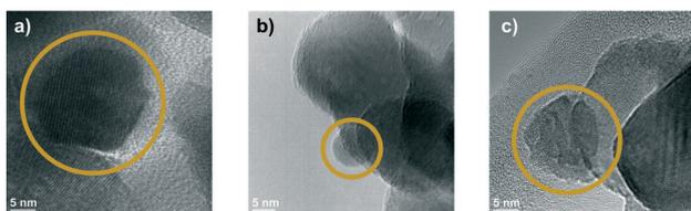
Fig. 1 TEM images of a) Ni-ZrO<sub>2</sub>, b) Cu-ZrO<sub>2</sub> and c) 11CuNi-ZrO<sub>2</sub>. The particles inside the circles were identified *via* EDX as Ni in a), Cu in b) and CuNi in c).
