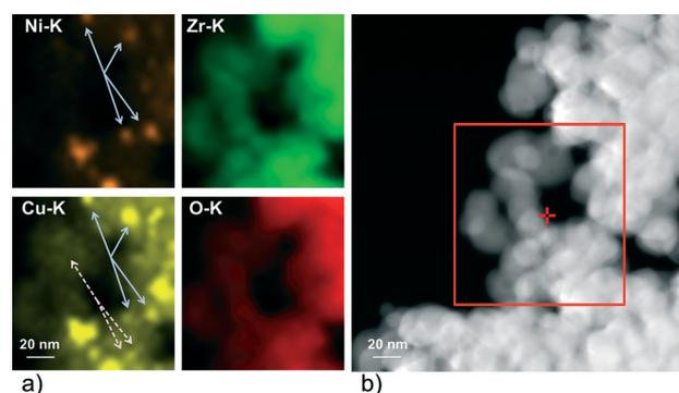
Fig. 2 a) Elemental map of the region shown in the rectangle in b) for the K edge energies of Ni, Cu, Zr and O recorded on 11CuNi-ZrO<sub>2</sub>. Full arrows: particles containing both Ni and Cu, dashed arrows: Cu but no Ni detected.
