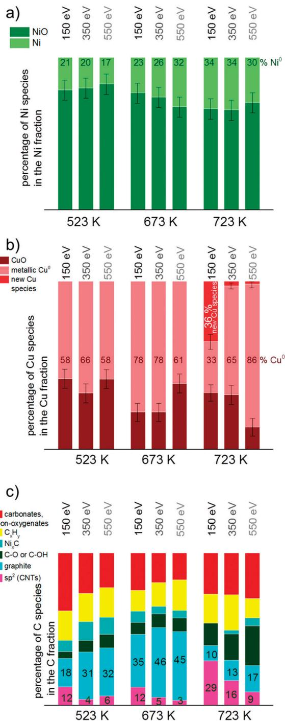
Fig. 9 Depth profile of a) Ni, b) Cu and c) C species based on the total amount of Ni, Cu and C, respectively. Spectra in the core level regions Ni 2p<sub>3/2</sub>, Cu 2p<sub>3/2</sub> and C 1s with kinetic energies of 150, 350 and 550 eV were consulted for the calculations. For clarity of the diagram error bars were left out in c).
