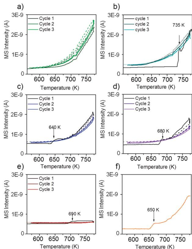
**Fig. 3** Hydrogen evolution during methane TPMd on a) Ni-ZrO<sub>2</sub>, b) 13CuNi-ZrO<sub>2</sub>, c) 11CuNi-ZrO<sub>2</sub>, d) 31CuNi-ZrO<sub>2</sub>, e) Cu-ZrO<sub>2</sub> and f) 13CuNi-ZrO<sub>2</sub>.50. The samples a)–f) were reduced at 673 K followed by 3 heating-cooling cycles between 573 and 773 K in methane/Ar. For f) only one heating cycle is shown. The temperature was ramped at 5 K min<sup>-1</sup>.
