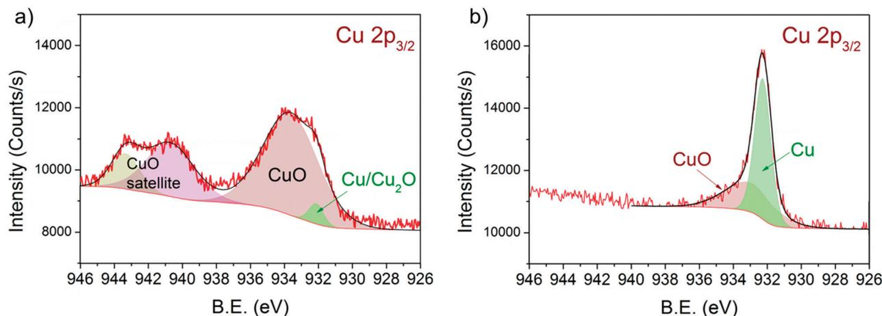
Fig. 5 Cu  $2p_{3/2}$  region of  $^{13}\text{CuNi-ZrO}_2$  50 in a) 0.10 mbar  $\text{O}_2$  at 573 K and b) 0.25 mbar  $\text{H}_2$  at 673 K for 30 min. The incident photon energy was 1100 eV.
