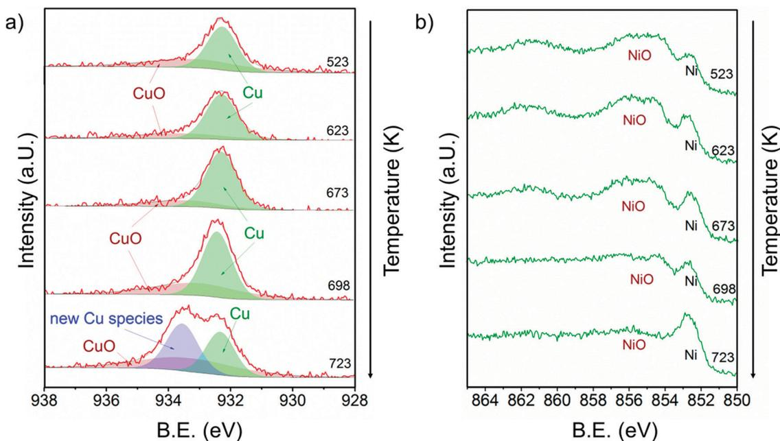
**Fig. 7** a) Cu 2p<sub>3/2</sub> and b) Ni 2p<sub>3/2</sub> core level regions of <sup>13</sup>CuNi-ZrO<sub>2</sub> in 0.25 mbar CH<sub>4</sub> at rising temperature from 523 to 723 K. The incident photon energies were 1100 eV (Cu) and 1010 eV (Ni).
