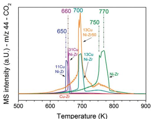
**Fig. 4** TPO performed after the methane decomposition reaction over Ni and all CuNi catalysts (shown in Fig. 3). The mass spectrometry trace of CO<sub>2</sub> (*m/z* 44) is displayed upon heating in 20 vol% O<sub>2</sub>/Ar at a rate of 5 K min<sup>-1</sup>.
