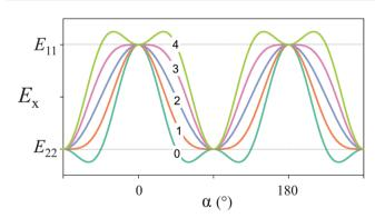
Fig. 7 Elastic modulus in the x-direction, according to eqn (4). We have taken  $E_{11}/E_{22} = 3$  (i.e. Young's modulus is three times larger in the direction of the fiber compared to perpendicular to the fiber axis) and the number (0 to 4) indicated for each graph corresponds to the value of  $(E_{12} + 2E_{66})/E_{22}$ (the shear contribution) inserted in the equation.
