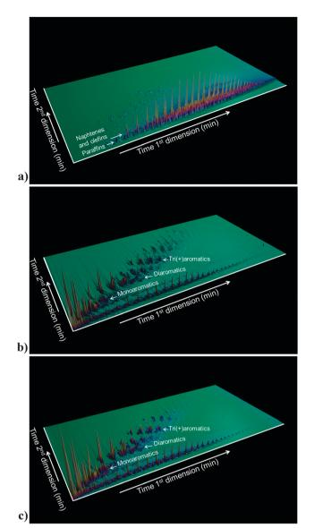
Fig. 5 (a) GC  $\times$  GC plot of a typical FCC feedstock (i.e., VGO). (b) GC  $\times$  GC plot of the products of cracking the VGO in (a), making use of an FCC catalyst with zeolite Y. (c) GC × GC plot of the products of cracking the VGO making use of an FCC catalyst with zeolite Y in the presence of zeolite ZSM-5 as additive.
