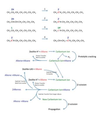
Fig. 9 Reaction network in zeolite-assisted cracking of hydrocarbon molecules. Reaction 1: proton transfer from zeolite Brønsted site to alkane to form carbonium ion. Reaction 2: proton transfer from zeolite to alkene to form carbenium ion. Reaction 3: hydride transfer from alkane to zeolite to form carbenium ion. Reaction 4: Beta scission of a carbenium ion to form a new carbenium ion and an alkene.
