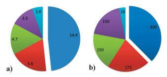
Fig. 1 (a) Installed capacities for the major conversion processes in refineries worldwide, in million barrels per day. (b) Number of refineries in which major conversion processes are installed. Refineries can have more than one technology installed. Data as of 2013, from ref. 1. Color-coding: fluid catalytic cracking (FCC): blue; hydrocracking: red; coking: green; thermal operations: purple; and resid hydrotreating: light blue.
