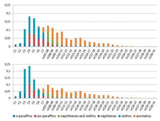
Fig. 15 A comparison of the total products from the same runs as depicted in Fig. 4. The graphs are combinations of the GC  $\times$  GC plot for total liquid product, PIANO analysis of the naphtha fraction, and GC analysis of the gases. Top: Products from a normal cracking run. Bottom: Products with ZSM-5 containing additive added to the catalyst. Colorcoding: n-paraffins: dark blue; iso-paraffins: red; naphthenes and olefins: green; naphthenes: purple; olefins: blue; aromatics: orange.
