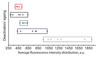
Fig. 29 Interparticle Brønsted acidity mapping for seven FCC1 catalyst particles, which have been subjected to different degrees of deactivation; *i.e.*, fresh, two-step cyclic deactivated (CD), Mitchell impregnated-steam deactivated (MI), and their comparison with the mapping results of seven E-cat catalyst particles. (Reproduced with permission from ref. 175, Copyright Macmillan Publishers. 2011).
