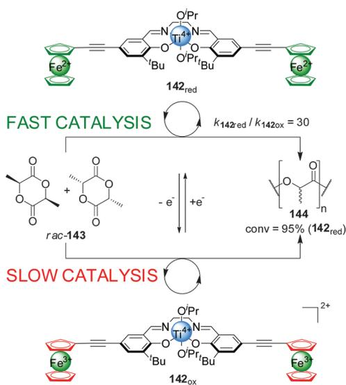
**Scheme 39** Influencing the rate of polymerization of *rac*-lactide (**143**) by oxidation/reduction of ferrocene groups pendant to a  $\text{Ti(IV)}$ –salen catalyst (**142**).<sup>71</sup>
