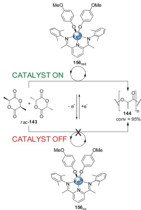
**Scheme 45** Iron-based redox-switchable catalyst **156** for the polymerization of *rac*-lactide.<sup>79</sup>
