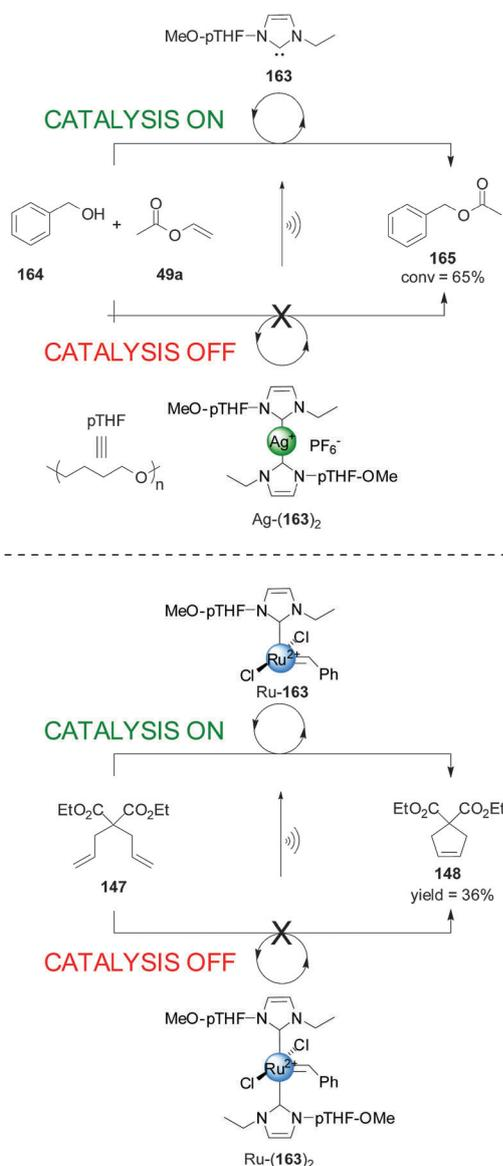
**Scheme 49** Polymer-functionalized catalysts activated by ultrasound-induced breaking of metal–ligand coordination bonds.<sup>87,88</sup>
