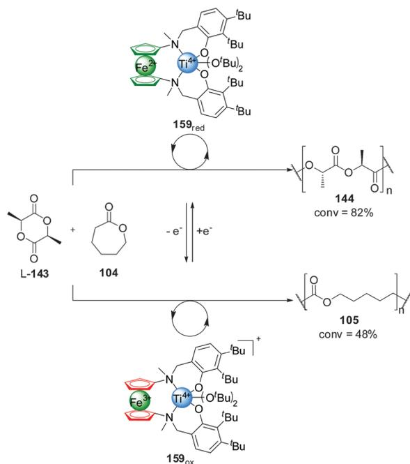
**Scheme 47** Switching of monomer selectivity by polymerization catalyst **159**, triggered by oxidation/reduction of the pendant ferrocene group.<sup>82</sup>
