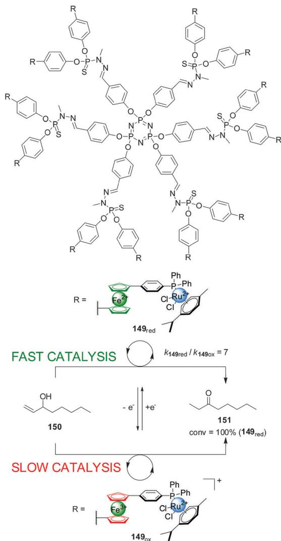
Scheme 42 Redox-switching of the rate of isomerization of allyl alcohol **150** using dendritic Ru(II)-catalyst **149**.<sup>75</sup>
