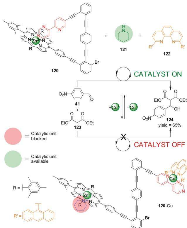
**Scheme 33** Switchable catalysis of a Knoevenagel reaction based on the capture/release of a piperidine catalyst (**121**) by Zn(II)–porphyrin **120** induced by the reversible coordination of Cu(I).<sup>64</sup>
