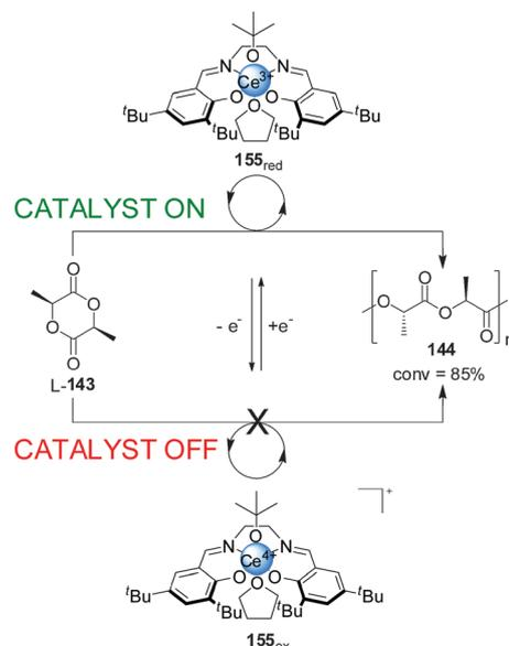
Scheme 44 'On-off' switching of lactide polymerization catalyst **155** triggered by reduction/oxidation of the cerium catalytic centre.<sup>77</sup>
