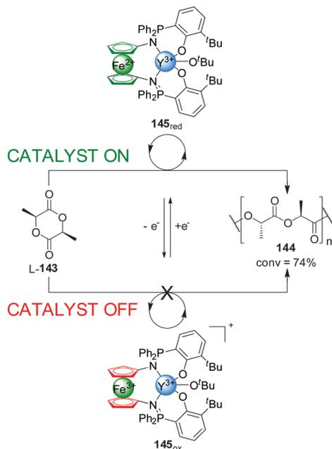
Scheme 40 'On-off' switching of catalyst **145** promoted by reversible ferrocene/ferrocenium redox reactions.<sup>72</sup>
