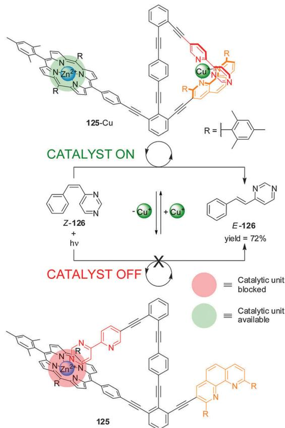
**Scheme 34** Control of the activity of catalyst **125** in a *cis-trans* isomerization process triggered by the addition/removal of Cu(I).<sup>65</sup>
