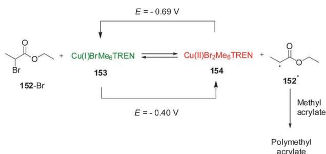
Scheme 43 Electrochemical control over the activation of a polymerization reaction by reduction/oxidation of Cu(I)/Cu(II).<sup>76</sup>
