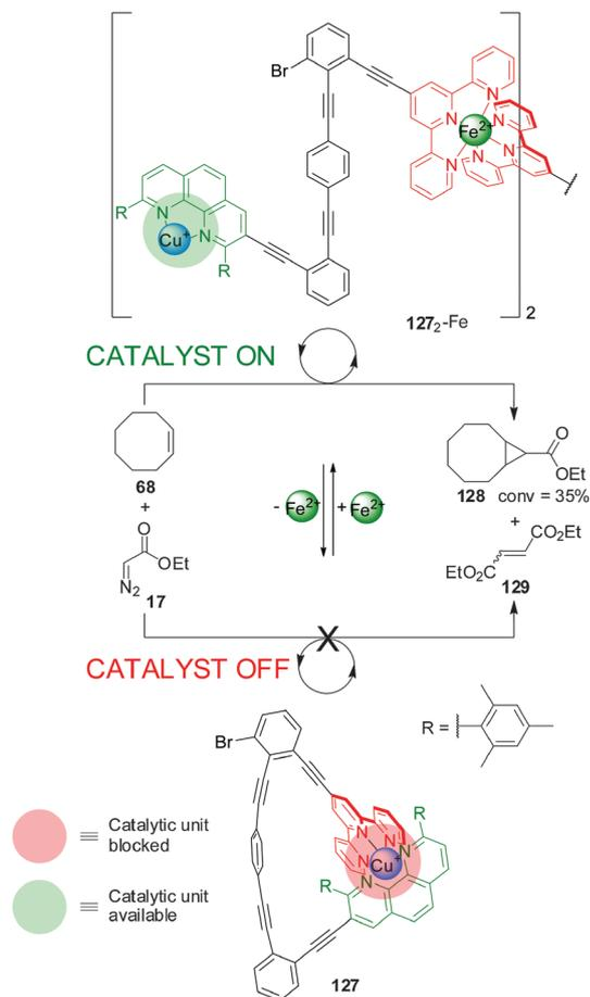
**Scheme 35** Control of the activity of Cu(I) catalyst **127** by switching between a monomeric and a dimeric form promoted by the reversible coordination of Fe(II).<sup>66</sup>
