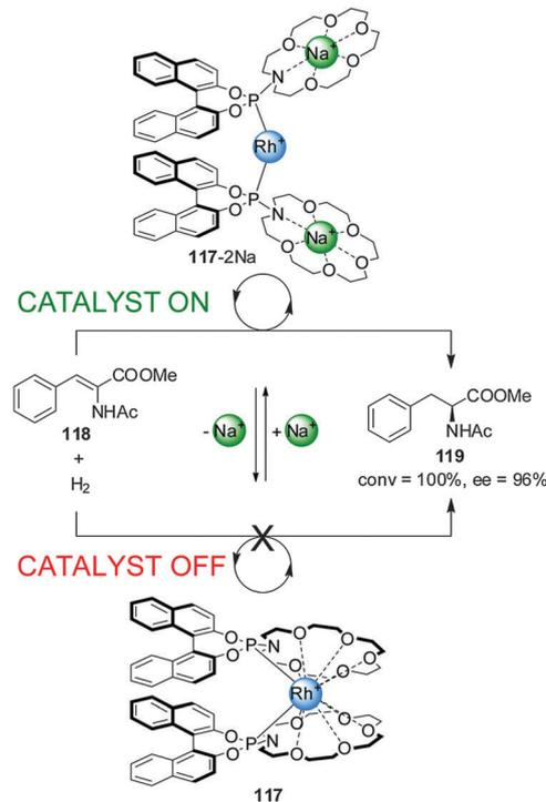
Scheme 32 'On-off' switching of Rh(I) catalyst **117** driven by addition or removal of Na<sup>+</sup> ions.<sup>63</sup>
