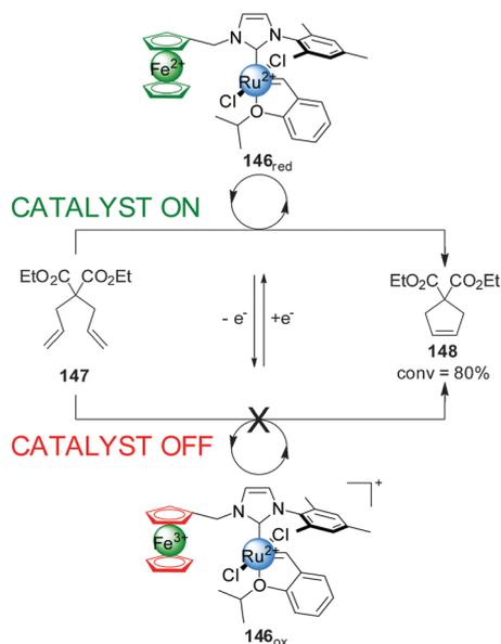
Scheme 41 Control over the activity of metathesis catalyst **146** by change of the oxidation state of a ferrocene iron centre.<sup>73</sup>
