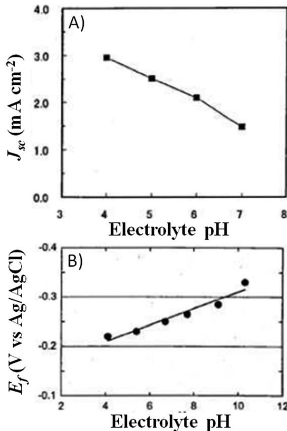
Fig. 18 (A) pH dependence of  $J_{sc}$  values ( $P_{in} = 1 \text{ sun}$ ) obtained for an aqueous DSSC sensitized with N719. Electrolyte: KI 0.50 M and  $I_2$  25 mM; (B) dependence of the Fermi level electrochemical potential ( $E_f$ ) of the mesoporous  $TiO_2$  electrode on the pH of the above reported electrolyte. The potential data were based on the measurement of the onset potential of dark cathodic current. Adapted and reprinted from ref. 138.
