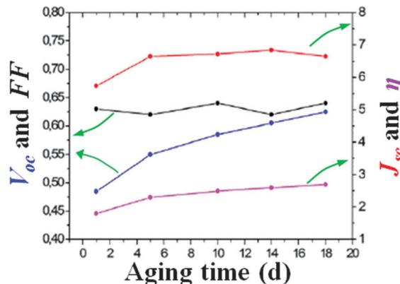
**Fig. 20** Long-term stability under dark of DSSCs assembled with a fully aqueous electrolyte (KI 4.0 M and  $\text{I}_2$  20 mM at pH 8.0) and a PEDOT counter electrolyte. Dye: V35. PV parameters were measured under  $P_{\text{in}} = 1$  sun. Adapted and reprinted from ref. 249.
