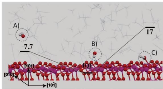
Fig. 8 Structures (with energy values in kcal mol<sup>-1</sup>) of the TiO<sub>2</sub>/bulk-ACN interfaces contaminated with water. (A) Water molecules exist in bulk ACN; (B) the most stable structure of water molecule in bulk ACN and water adsorbed on the TiO<sub>2</sub> surface *via* a hydrogen bond through the H atom in water; (C) water adsorbed onto the TiO<sub>2</sub> surface *via* a hydrogen bond through the O atom in water. Adapted and reprinted from ref. 108.
