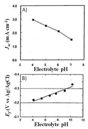
Fig. 18 (A) pH dependence of  $J_{sc}$  values ( $P_{in}=1$  sun) obtained for an aqueous DSSC sensitized with N719. Electrolyte: KI 0.50 M and I $_2$  25 mM; (B) dependence of the Fermi level electrochemical potential ( $E_f$ ) of the mesoporous TiO $_2$  electrode on the pH of the above reported electrolyte. The potential data were based on the measurement of the onset potential of dark cathodic current. Adapted and reprinted from ref. 138.
