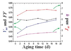
Fig. 20 Long-term stability under dark of DSSCs assembled with a fully agueous electrolyte (KI 4.0 M and I<sub>2</sub> 20 mM at pH 8.0) and a PEDOT counter electrolyte. Dye: V35. PV parameters were measured under  $P_{in} = 1$ sun. Adapted and reprinted from ref. 249
