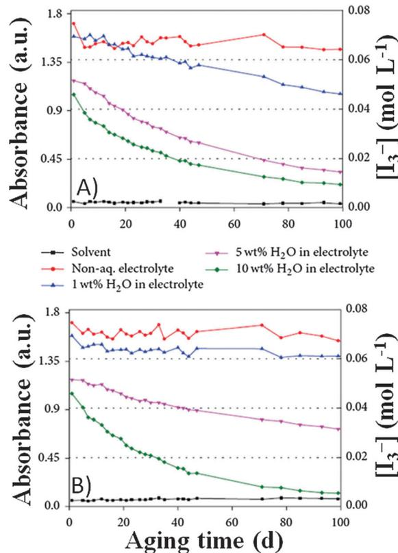
Fig. 22 Absorbance at 430 nm as a function of the aging time for DSSCs filled with solvent, non-aqueous electrolyte and redox electrolyte encompassing 1, 5 and 10 wt%  $\text{H}_2\text{O}$ , in the presence of different GFs as sealants: (A)  $\text{Bi}_2\text{O}_3\text{-SiO}_2\text{-B}_2\text{O}_3$ ; (B)  $\text{ZnO-SiO}_2\text{-Al}_2\text{O}_3$ . Adapted and reprinted from ref. 290.
