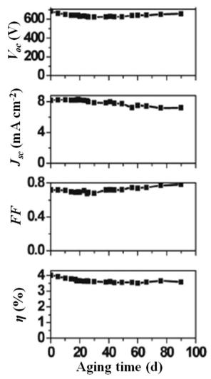
Fig. 14 Long-term stability under dark of a DSSC assembled with an aqueous electrolyte composed of  $[Co(bpy)_3]^{2+}$  0.20 M,  $[Co(bpy)_3]^{3+}$  40 mM, NMBI 0.70 M and PEG 300 1 vol%. Dye: MK-2. Adapted and reprinted from ref. 194.
