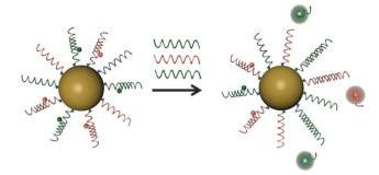
Fig. 10 Schematic representation of target detection of mRNA by multiplexed nanoflares. The multiplexed nanoflares bind different target nucleic acids (shown in red and green), displacing the corresponding flare. Once the flare is released, the fluorophore is no longer quenched by the gold surface, and an increase in fluorescence can be measured. Using two different fluorophores, the ratio of each target can be determined in cells. From ref. 233 with permission (2014) by the Am. Chem. Soc
