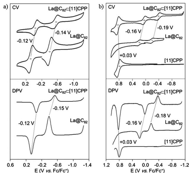
Fig. 105 Electrochemical behaviour of  $\text{La@C}_{82}\text{@[11]CPP}$ ,  $\text{La@C}_{82}$ , and [11]CPP. Cyclic voltammograms and differential pulse voltammograms of  $\text{La@C}_{82}\text{@[11]CPP}$ ,  $\text{La@C}_{82}$ , and [11]CPP are shown in (a) *ortho*-dichlorobenzene and (b) nitrobenzene with  $\text{Bu}_4\text{NPF}_6$ . Reproduced with permission from ref. 117. Copyright 2014 Wiley-VCH Verlag GmbH & Co. KGaA, Weinheim.
