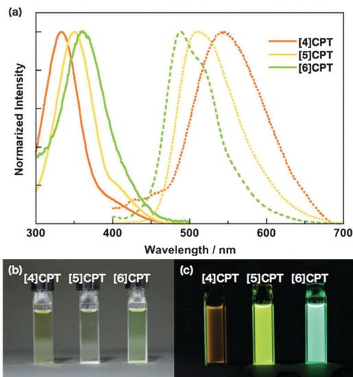
**Fig. 116** (a) UV-vis absorption (broken line) and fluorescence spectra (solid line) of **[4]CPT**, **[5]CPT**, and **[6]CPT** in cyclohexane (absorption and fluorescence spectra were normalized). (b) Pictures of **[4]CPT**, **[5]CPT**, and **[6]CPT** in cyclohexane under (b) ambient light and (c) UV irradiation at 365 nm. Reproduced with permission from ref. 123. Copyright 2015 Wiley-VCH Verlag GmbH & Co. KGaA, Weinheim.
