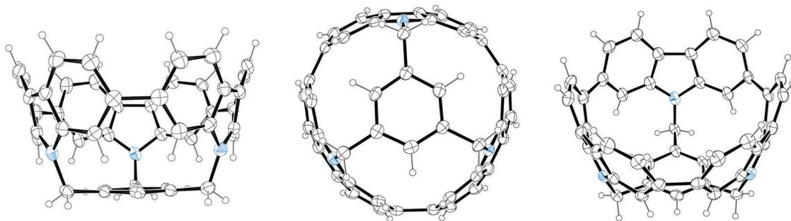
Fig. 119 ORTEP diagram showing three views of **300** (one of three molecules in the unit cell), showing ellipsoids at 30% probability. H atoms are shown as spheres of arbitrary radius. Solvent has been omitted for clarity.
