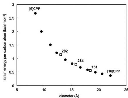
Fig. 112 Strain energies of carbon nanocages **131**, **282** and **284** (square) and [6]–[16]CPP (filled circle) per carbon atom versus diameters (B3LYP/6-31G(d)). Adapted with permission from ref. 122. Copyright 2014 American Chemical Society.
