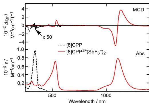
Fig. 117 Magnetic circular dichroism (top) and electronic absorption (bottom) spectra of [8]CPP<sup>2+</sup>(SbF<sub>6</sub><sup>-</sup>)<sub>2</sub> (red solid line) and [8]CPP (black broken line) in CH<sub>2</sub>Cl<sub>2</sub> at room temperature under Ar. Reproduced with permission from ref. 124. Copyright 2015 American Chemical Society.
