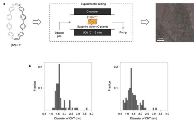
Fig. 59 (a) Schematic representation of experimental setup for Itami's synthesis of carbon nanotubes from CPPs; TEM image of nanotubes synthesised from [12]CPP. (b) Nanotube diameter distribution histograms for [12]CPP (left) and [9]CPP (right). Reproduced with permission from ref. 78. Copyright 2013 Nature Publishing Group.
