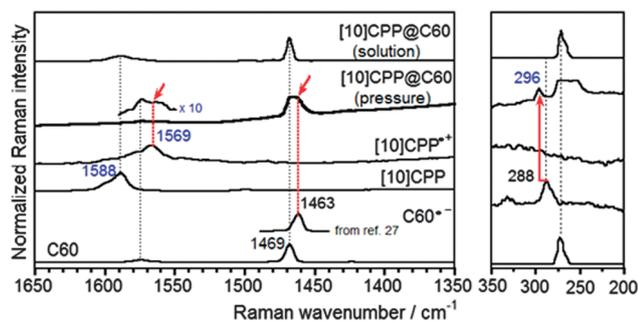
Fig. 96 785 nm Raman spectra of 1:1 CHCl<sub>3</sub> solution mixtures of [10]CPP and C<sub>60</sub> and in solid state after the application of a 6 GPa pressure. The spectra of the neutral C<sub>60</sub> and [10]CPP together with those of the C<sub>60</sub> anion and of the CPP radical cation are also shown. Reproduced with permission from ref. 109. Copyright 2014 Wiley-VCH Verlag GmbH & Co. KGaA, Weinheim.
