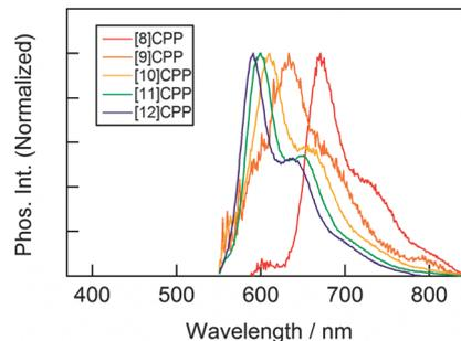
Fig. 97 Normalized phosphorescence spectra of [n]CPP (n = 8–12) in EET solvent at 77 K. Excited at 350 nm. Phosphorescence spectra were measured by applying gate between 50  $\mu$ s and 1 ms after excitation. Reproduced with permission from ref. 110. Copyright 2014 American Chemical Society.
