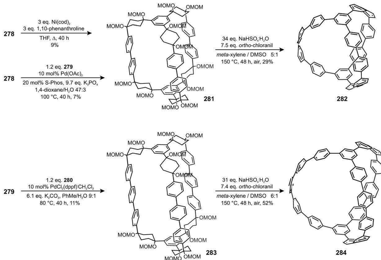
Scheme 59 Synthesis of carbon nanocage Y-branching units **282** and **284**.
