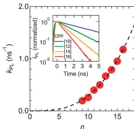
Fig. 86 The photoluminescence decay rate,  $k_{PL}$ , at room temperature as a function of the number of benzene rings,  $n$ . The inset shows the photoluminescence decay curves of the  $[n]$ CPPs ( $n = 10, 12, 14, 16$ ). Reproduced with permission from ref. 102. Copyright 2014 Royal Society of Chemistry.
