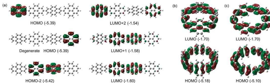
Fig. 93 HOMO and LUMO of (a) tetra-2,7-pyrene, (b) [4]CPY, and (c) [8]CPP. Orbital energies (in eV) calculated at the B3LYP/6-31G\* level of theory are shown in parentheses. Reproduced with permission from ref. 108. Copyright 2014 Wiley-VCH Verlag GmbH & Co. KGaA, Weinheim.
