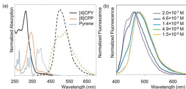
Fig. 94 (a) UV/visible absorption and fluorescence spectra of the solutions of [4]CPY, [8]CPP and pyrene in CHCl<sub>3</sub>. (b) Concentration-dependent fluorescence of [4]CPY in CHCl<sub>3</sub>. The fluorescence spectra were obtained by exciting the sample at  $\lambda = 370$  nm. Reproduced with permission from ref. 108. Copyright 2014 Wiley-VCH Verlag GmbH & Co. KGaA, Weinheim.
