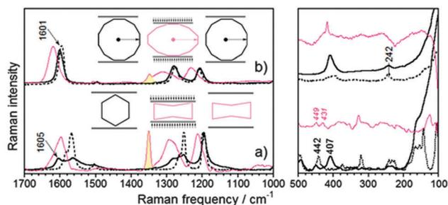
Fig. 95 785 nm Raman spectra of: (a) [6]CPP and (b) [12]CPP, before (dotted line), with an applied pressure around 6 GPa (pink line) and after the pressure release (solid line). Inset diagrams represent (from left to right) the molecular models before applied pressure, with applied pressure, and after release. Reproduced with permission from ref. 109. Copyright 2014 Wiley-VCH Verlag GmbH & Co. KGaA, Weinheim.
