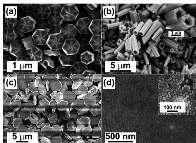
Fig. 10 SEM characterization of lanthanide-doped UC crystals. (a) Flower-patterned hexagonal plates of  $\text{NaYF}_4$ . (b)  $\text{NaYbF}_4:\text{Tm}$  (1.0 mol%) microtubes. (c)  $\text{NaYbF}_4$  microplates (unpublished result). (d)  $\text{NaYF}_4:\text{Yb}/\text{Er}$  (20/2 mol%) nanocrystal assemblies. (Reprinted with permission from ref. 106, 145 and 147. Copyright 2007, 2010, 2011 and 2009, Wiley-VCH Verlag GmbH & Co. KGaA, American Chemical Society and Royal Society of Chemistry.)
