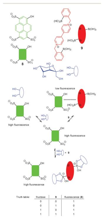
Fig. 6 Chemical principles of the sugar computer and the IMPLICATION truth table. Adapted from ref. 20 with permission from Wiley
