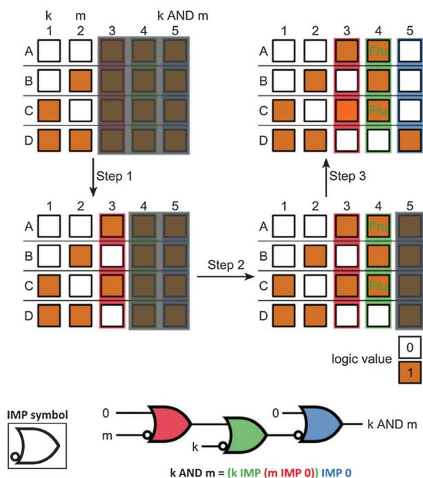
Fig. 7 Algorithm-based titration protocol for the concatenation of molecular IMPLICATION gates. Adapted from ref. 20 with permission from Wiley.
