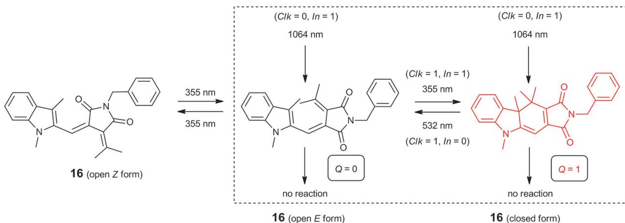
Fig. 10 Photochromic switching of fulgimide **16** for the realization of a D flip-flop.
