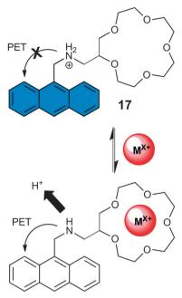
Fig. 12 pK<sub>a</sub>-Shift and the resulting PET switching induced by cation complexation to the crown ether.
