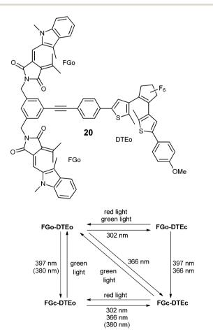
Fig. 15 Structure of the all-open isomeric form of the FG-DTE multitasking triad 20 (top) together with the corresponding isomerization scheme (bottom)
