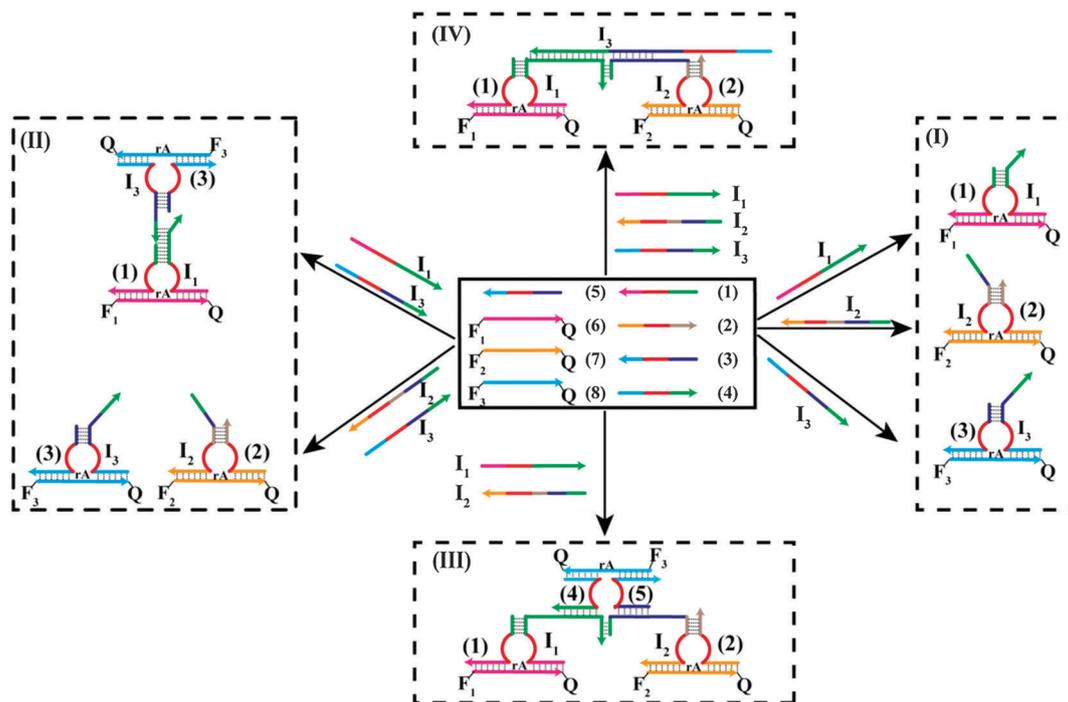
Fig. 16 Single-stranded oligonucleotide library (1–8) and the corresponding input strands ( $I_1$ – $I_3$ ) for the Toffoli gate. The bulge-like DNAzyme structures induce strand breaks, which in turn switch on the fluorescence from  $F_1$ – $F_3$ . Reproduced from ref. 45.
