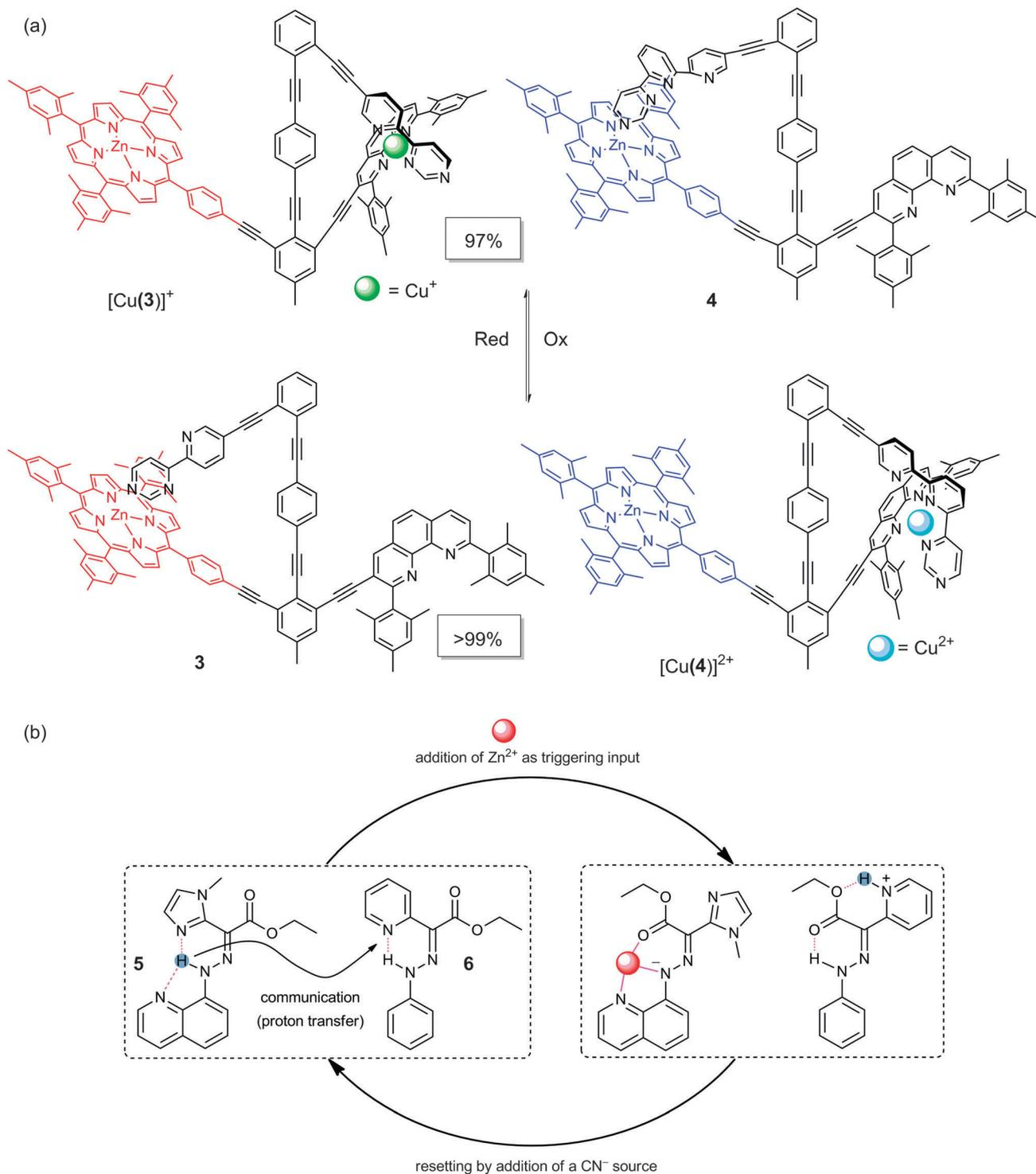
Fig. 4 Switch-to-switch communication by (a) redox chemistry and (b) coordination-coupled deprotonation. (a) was adapted from ref. 13 with permission from Wiley.
