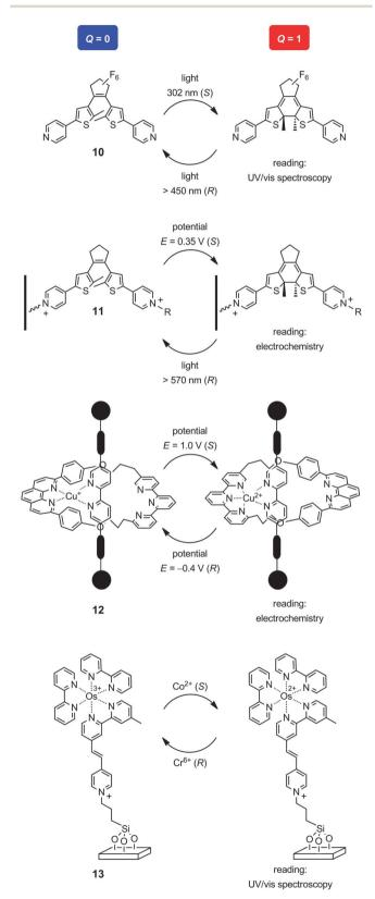
Fig. 8 Examples for molecular set-reset flip-flops.
