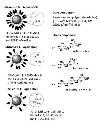
Fig. 15 PEI-OS architectures and analytes used in the study by B. Voit and co-workers. Top: the investigated PEI-OS architectures are shown with the three types of oligosaccharides, Mal, Lac, Mal-III, that act as shell components and with two PEI cores, PEI-5k and PEI-25k. The various substructures A, B, and C and the differences in their oligosaccharide shell densities are also illustrated. Reprinted from ref. 78; Copyright 2014, with permission from WILEY-VCH.
