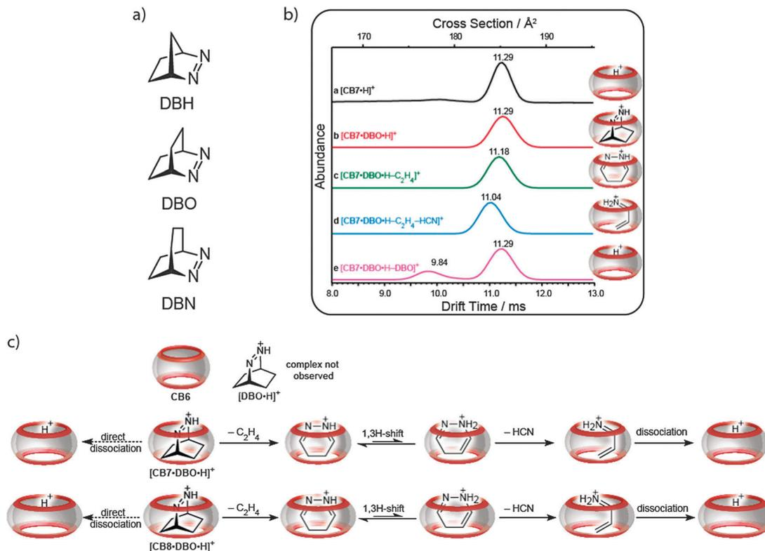
Fig. 23 (a) Chemical structures of the bicyclic azoalkanes. (b) Ion mobilograms of different CB7 complexes. (c) Reaction and dissociation pathways of the inclusion complex of DBO inside CB<sub>n</sub> in the gas phase.
