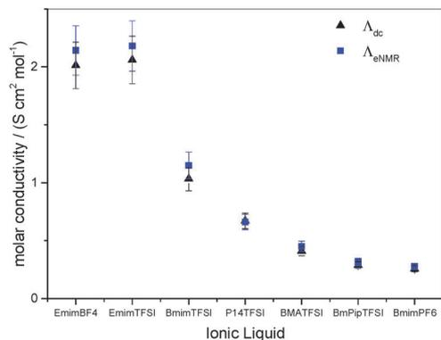
Fig. 3 Molar conductivity  $\Lambda_{dc}$  determined by impedance spectroscopy (black triangles) compared with the molar conductivity  $\Lambda_{eNMR}$  (blue squares) calculated from electrophoretic mobilities at 295 K. Errors are estimated to  $\pm 10\%$ .
