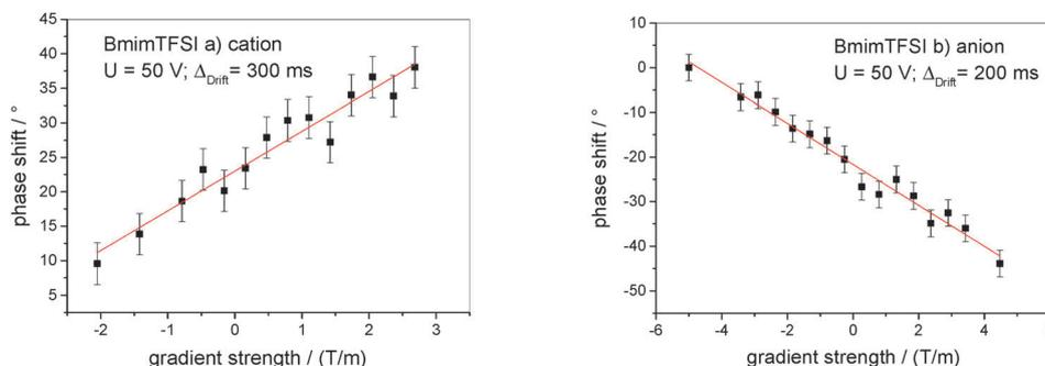
Fig. 1 Phase shift in dependence on the gradient strength of BmimTFSI for (a) cation (<sup>1</sup>H) and (b) anion (<sup>19</sup>F). Errors are estimated to  $\pm 3^\circ$ . The red line follows from a linear regression.
