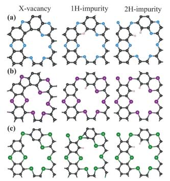
Fig. 5 Optimized X-vacancy and their H substituted structures of (a) C<sub>2</sub>N, (b) C<sub>2</sub>P, and (c) C<sub>2</sub> As respectively.
