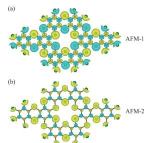
Fig. 3 Charge density difference,  $\rho_{up} - \rho_{down}$ , of the C<sub>2</sub>As monolayer structure for (a) fully anti-ferromagnetic (AFM-1) order and (b) antiferromagnetic order in the benzene ring (AFM-2) where green/yellow color is for minority/majority spin states. The plotted isosurface values are  $10^{-3}$  e Å<sup>-3</sup> and  $10^{-5}$  e Å<sup>-3</sup> for (a) and (b) respectively.
