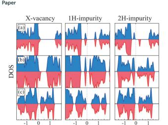
Fig. 6 Total DOS for defected and H-impurity structures of (a) C<sub>2</sub>N, (b) C<sub>2</sub>P, and (c) C<sub>2</sub>As respectively.
