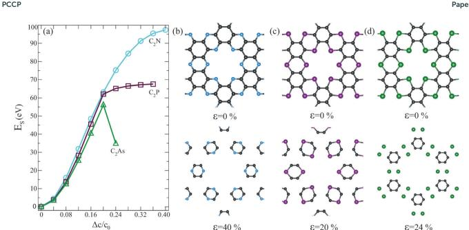
Fig. 4 (a) Change in total energy of the three holey graphene monolayers under applied strain. Structural changes under applied strain of (b) C<sub>2</sub>N, (c) C<sub>2</sub>P and (d) C<sub>2</sub>As.
