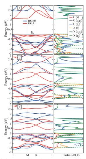
Fig. 2 Band-structures (left-panel) and corresponding partial density of states (right-panel) of (a)  $C_2N$ , (b)  $C_2P$ , and (c)  $C_2As$  where red curves are for bands calculated within GGA approximation while dashed blue curves are for bands calculated within HSE06 on top of GGA. The Fermi energy  $(E_{\varepsilon})$  level is set to the valence band maximum
