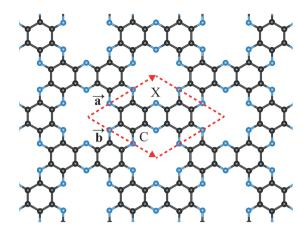
Fig. 1 Top view of the C<sub>2</sub>X holey graphene monolayer structure where X represents N, P or As atoms.
