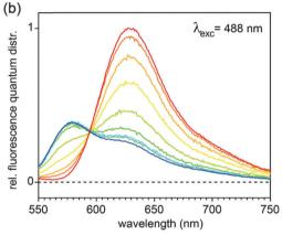
Fig. 1 Optical absorption (a) and fluorescence (b) spectra of PAc–SNARF in water/dmso (20:1 by volume, for buffer see text) as function of pH at 22 °C. Red and blue curves represent the species-associated spectra (SAS) of the pure deprotonated and protonated species, respectively, from global analysis. In stationary measurements, excitation wavelength  $\lambda_{\rm exc}=488$  nm was chosen in order to enhance the fluorescence contribution by the protonated species.
