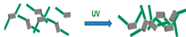
Fig. 12 Proposed model of the H8-azo-H8 monolayer at the air-water interface before and after exposure to UV light.
