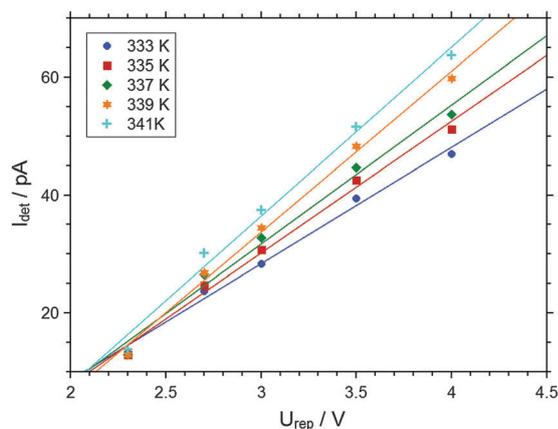
Fig. 5 Temperature dependent current–voltage characteristics of (PAH/PSS)<sub>12</sub>.
