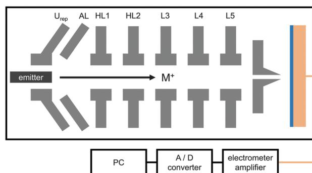
Fig. 2 Setup for BIIT experiments with the repeller lens  $U_{\text{rep}}$ , the abstraction lens AL, and five lenses; HL1, HL2 allow adjusting the direction of the ion beam, lenses L3–L6 are used for refocusing the ion beam ensuring a homogeneous beam profile.
