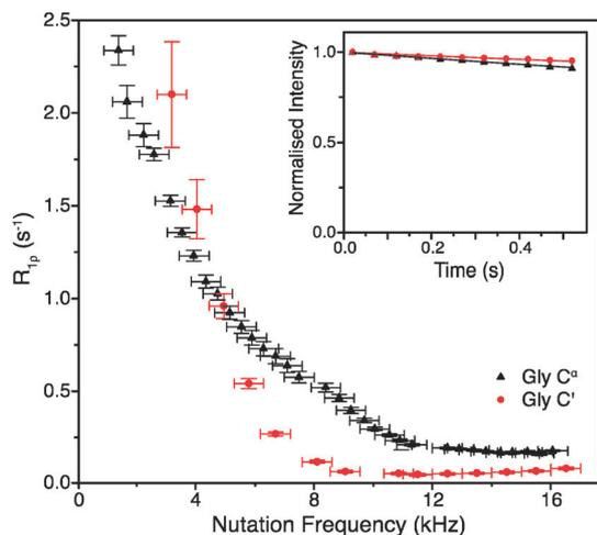
Fig. 1  $R_{1\rho}$  dispersion for  $^{13}\text{C}'$  (red circle) and  $^{13}\text{C}^\alpha$  (black triangle) in  $[\text{U-}^{13}\text{C},^{15}\text{N}]$ glycine at  $\omega_{\text{OH}}/2\pi = 600$  MHz,  $\omega_r/2\pi = 60$  kHz, and (inset) example  $R_{1\rho}$  decay curves for with  $\omega_1/2\pi = 17$  kHz.
