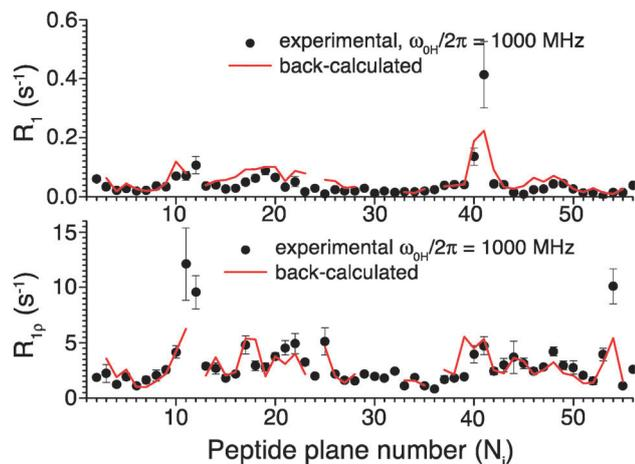
Fig. 6 Comparison of  $^{15}\text{N}$   $R_1$  and  $R_{1p}$  relaxation rates measured in crystalline GB1 at 1 GHz  $^1\text{H}$  Larmor frequency (black points)<sup>4</sup> and those back-calculated from an EMF analysis based on  $^{15}\text{N}$  and  $^{13}\text{C}'$  relaxation rates measured at 600 and 850 MHz  $^1\text{H}$  Larmor frequencies in Fig. 5 (red line).
