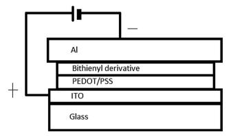
Fig. 1 OLED structure with the details of the organic materials and their functions used in each layer.
