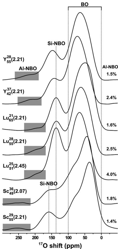
Fig. 1 <sup>17</sup>O NMR spectra recorded from the as-indicated RE<sub>2</sub>O<sub>3</sub>-Al<sub>2</sub>O<sub>3</sub>-SiO<sub>2</sub> glasses at 14.1 T and 24.0 kHz MAS. The signals from BO and Si-NBO moieties are marked by dotted lines, whereas that from Al-NBO is highlighted by a grey rectangle. The relative amounts (in %) of the Al-NBO moieties out of the entire O speciation is indicated at the right portion of each spectrum.
