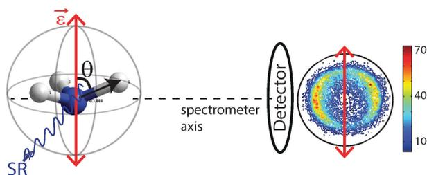
Fig. 2 Geometry of experimental setup:  $\theta$  is the angle between the polarisation vector,  $\vec{\varepsilon}$ , and the broken molecular bond.  $\vec{\varepsilon}$  is perpendicular to the propagation direction of synchrotron radiation (SR) and spectrometer axis. The expected alignment of  $NH_3$  relative to  $\vec{\varepsilon}$  for the  $N1s \rightarrow 4a_1$  transition is indicated. Example of a detector image is included showing perpendicular ejection of  $H^+$  fragment.
